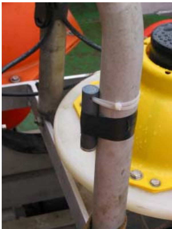
Figure 5.1e. Vemco minilog attached to ADCP frame
