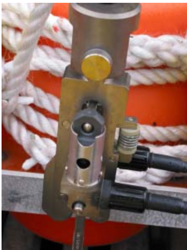
Figure 5.1d. Titanium release and “fizz link”
