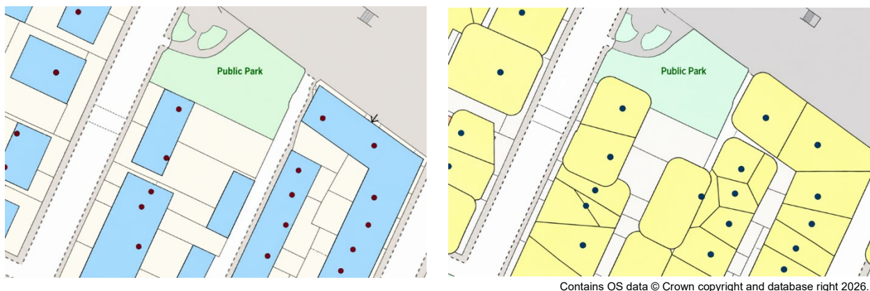
Figure 5 Examples of UPRN footprint processing (Left) and Voronoi-based subdivision of a building footprint containing multiple UPRNs (Right).
