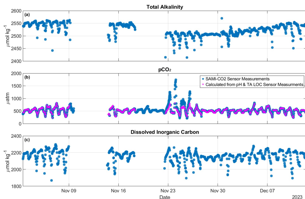
Figure 5. Time series of carbonate system observations on the Cement Wreck back reef. (a) total alkalinity (TA) in \mu\text{mol kg}^{-1} , (b) p\text{CO}_2 (in \mu\text{atm} ) measured by the SAMI-CO2 sensor (blue) and p\text{CO}_2 derived from pH and TA LOC sensor measurements (pink) (c) derived dissolved inorganic carbon (DIC) in \mu\text{mol kg}^{-1} are plotted from 02 November–12 December 2023. Gaps in timeseries reflect sensor downtime (a–b) and therefore corresponding missing derived DIC (c) and derived p\text{CO}_2 (b).
