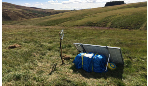
Underline differential magnetometer system in-situ at Whiteadder, Scottish Borders
