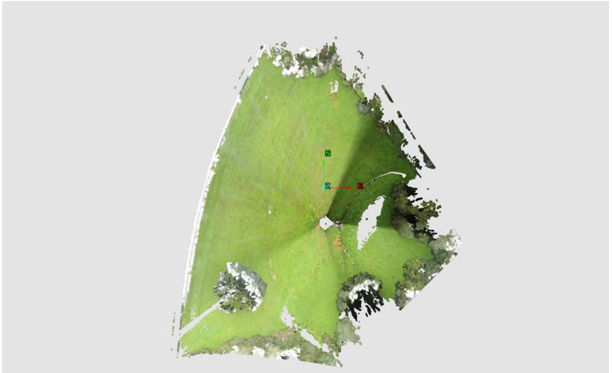
Figure 12 – Point cloud of Dam generated from Riegl VZ-1000 scan
