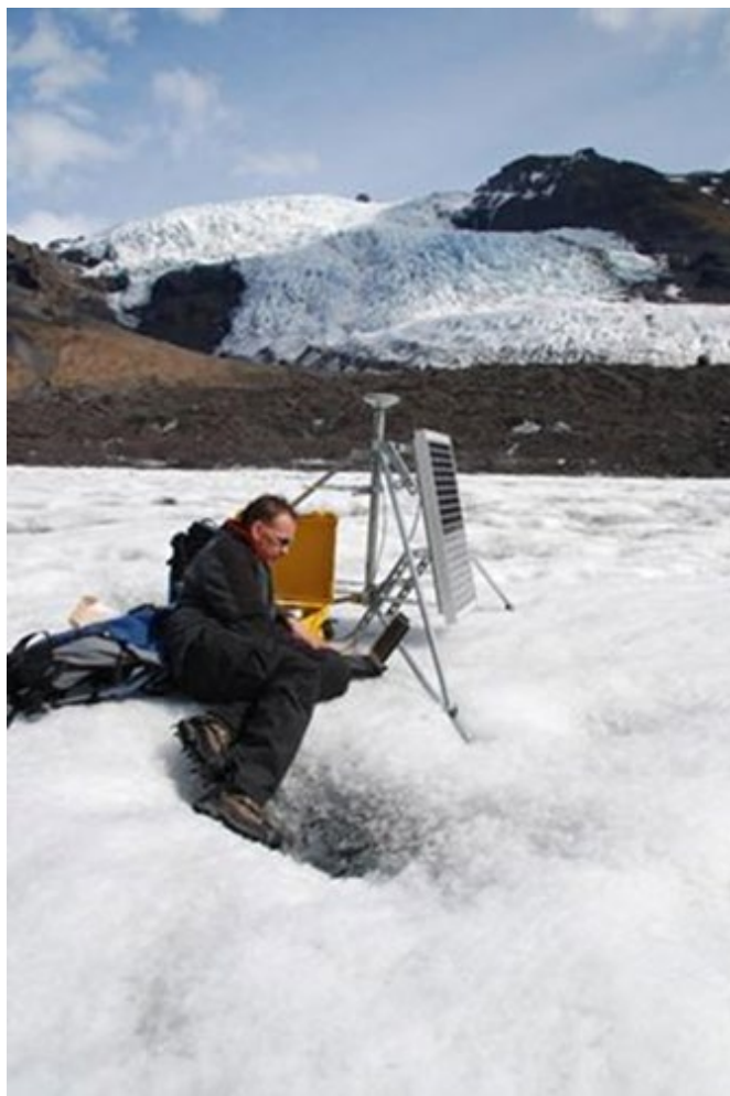
Figure 3 – GS10 system acting as on-ice ground control at Virkisjokull, Iceland
