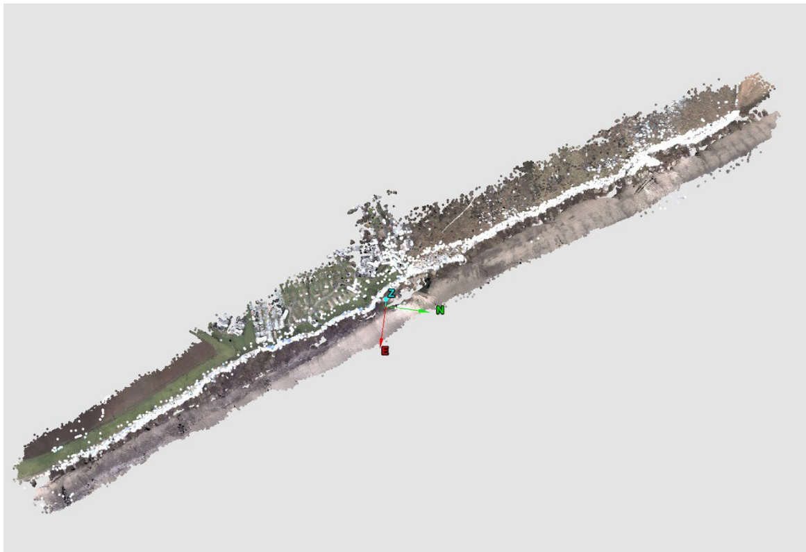
Figure 27 – Point cloud of Cliff top generated from Pegasus walk-over survey
