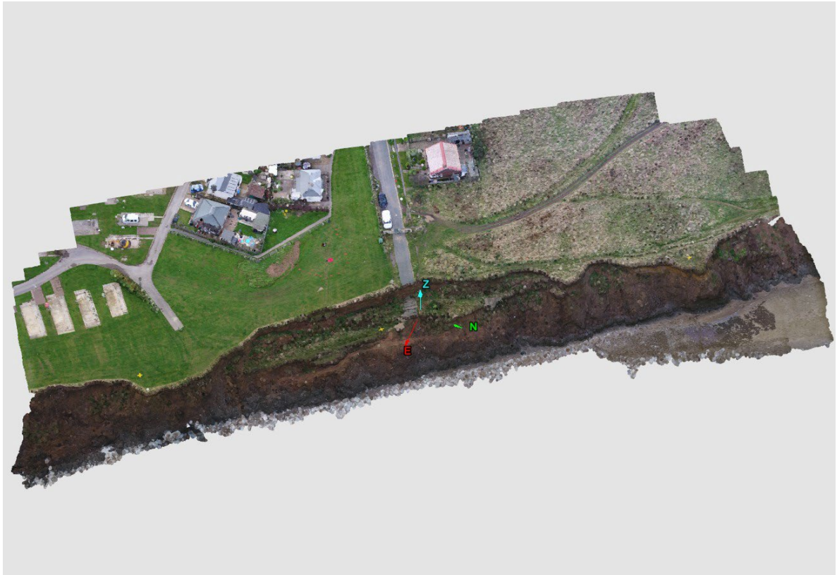
Figure 30 – Point cloud generated from DJI M210RTK oblique photogrammetric image
