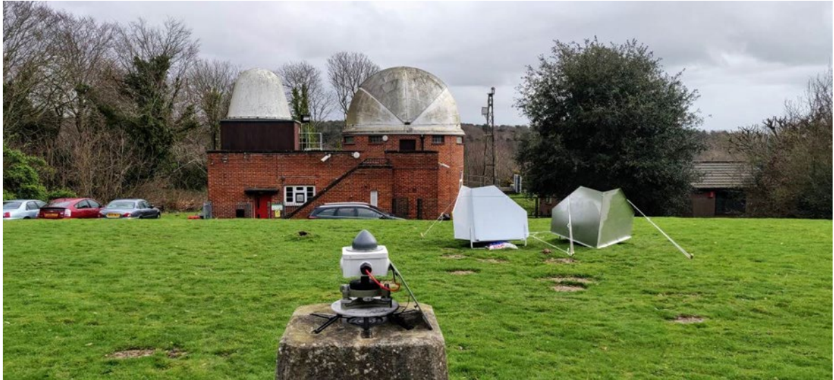
Figure 7 – Low Cost GNSS unit on OS Trig. Point at Herstmonceux. Sussex
