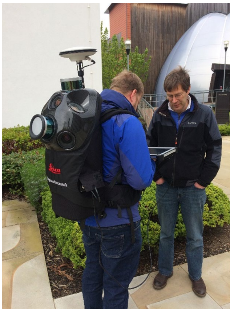
Figure 2 - Leica Pegasus Backpack Mobile Mapping Solution
