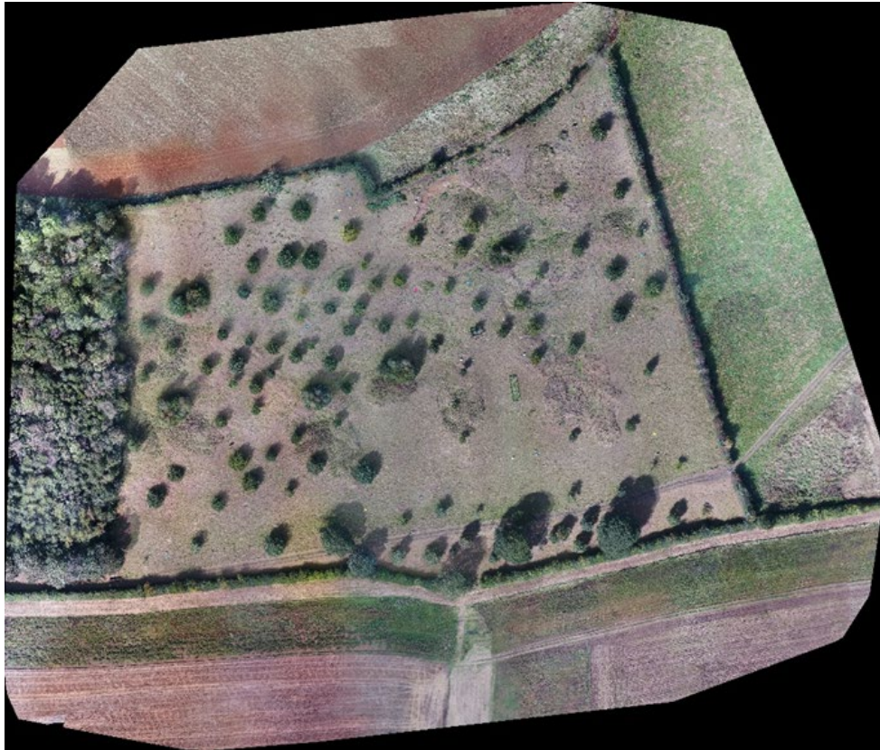
Figure 22 – Photogrammetric image generated from DJI Matrice 210RTK UAV
