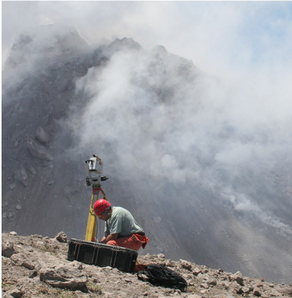
Figure 5 – Scanning the active lava dome of the Soufrière Hills Volcano, Montserrat
