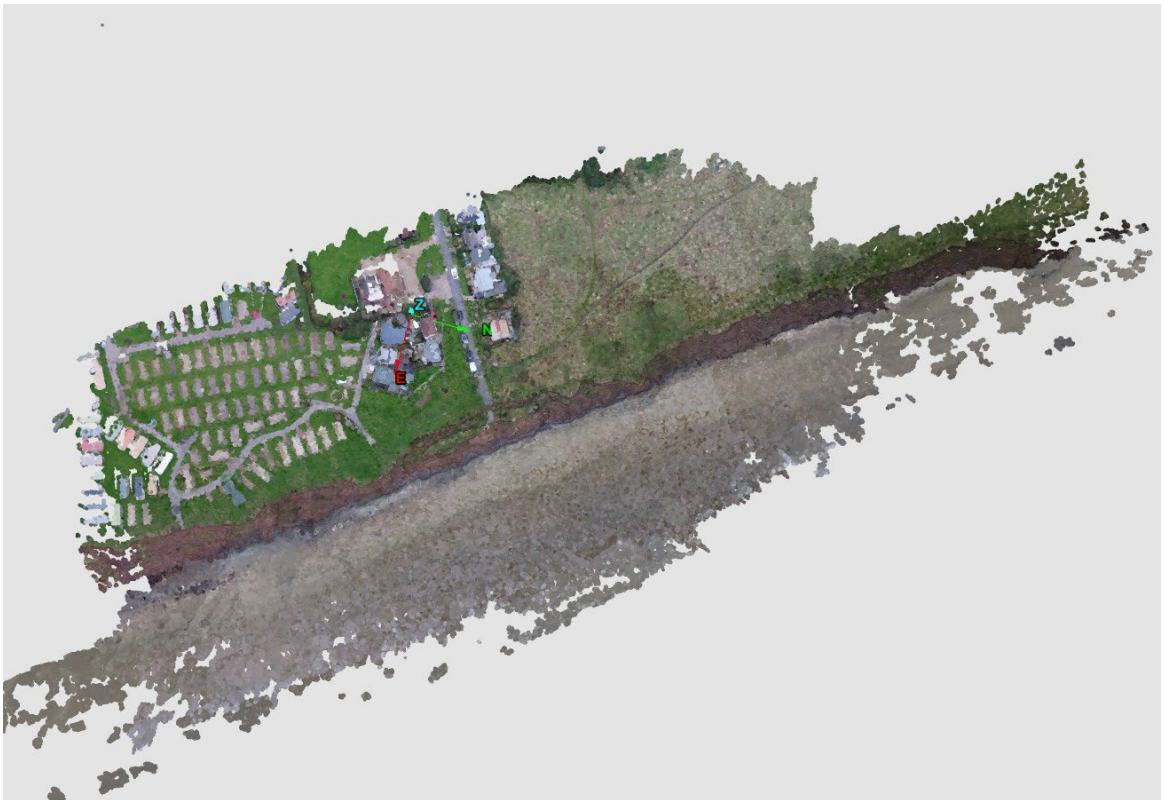
Figure 29 – Point cloud generated from DJI M210RTK photogrammetric image
