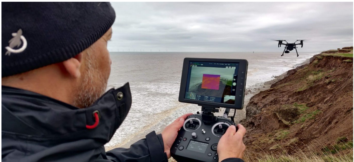
Figure 8 – DJI M210 with thermal camera at Aldbrough, Yorkshire
