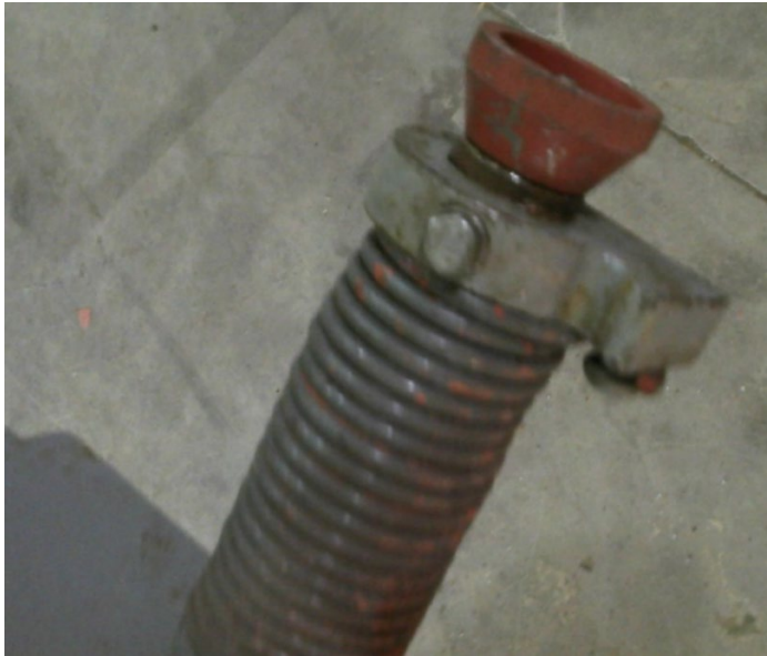
Figure 15: This shows the red pins flush to their mounting, this suggests the bucket is securely in place.
