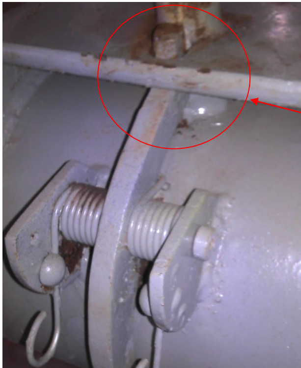
Figure 17: This shows the pawl engagement, locking the bucket in place.
