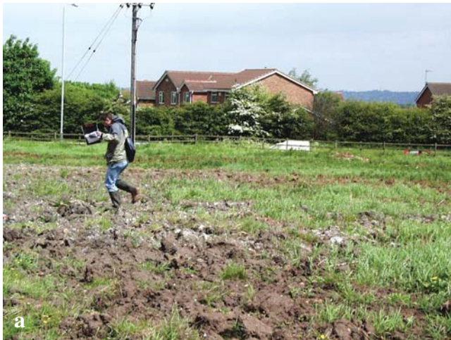
Figure 6.21 Soil disturbances over mineshafts at Chilwell Dam Farm, (NGR 451430, 42890).
