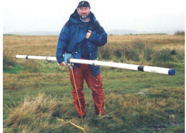
Figure 6.4 Geonics EM 31 system with an inter-coil spacing of 3.66 metres.
