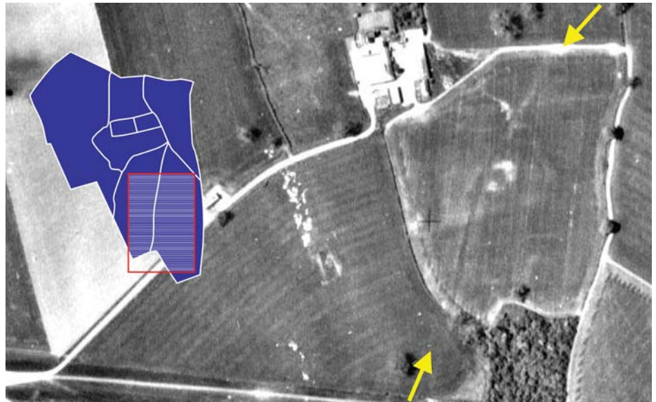
Figure 4.6 Tonal contrast within a conventional black and white aerial photograph were useful indicators of disused workings. The track of the Kimberly Colliery Tramway is indicated between two arrows whilst the remnants of other man-made features are also visible.
