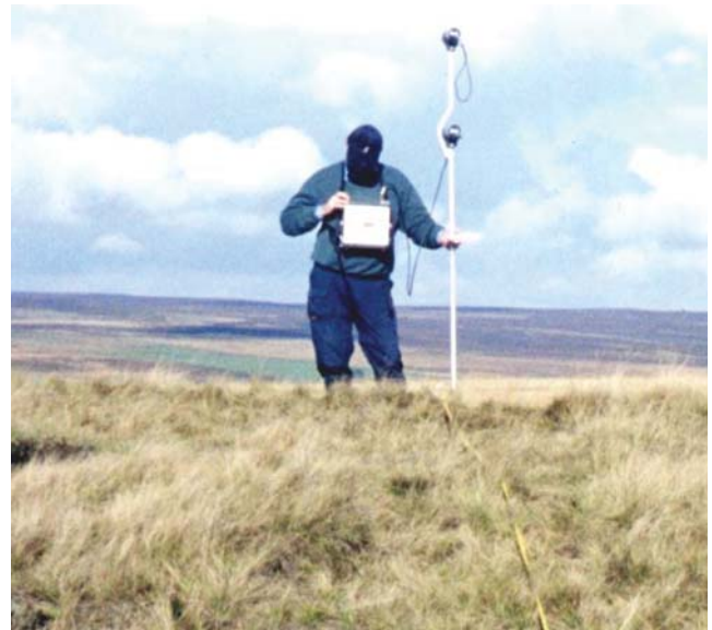
Figure 6.7 The Scintrex IG-2 field magnetometer equipment. (The staff has two proton precession units at approximately 1.5 m and 2.0 m above the ground.)
