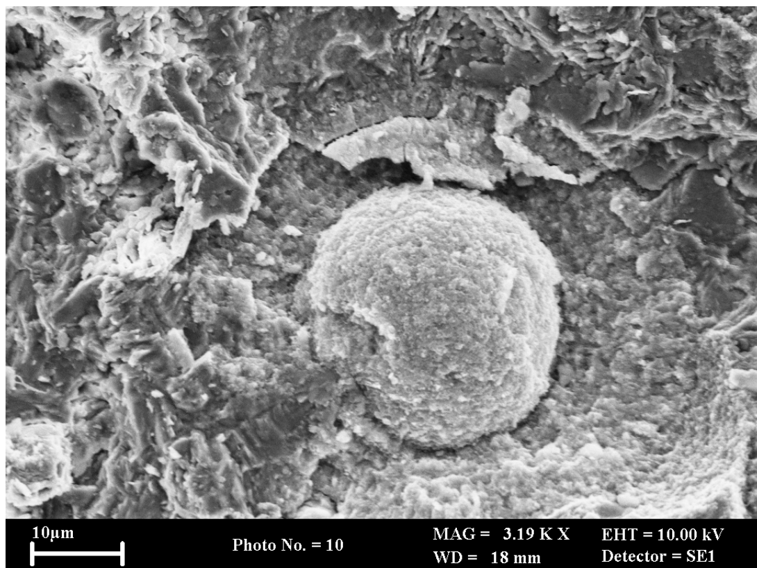
Plate 7. Scanning electron photomicrograph showing a higher magnification view of the internal fibro-radial structure of a fractured Mn oxyhydroxide/gibbsite sphere.
