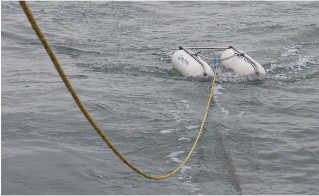
Figure 25 BGS surface tow boomer (STB) deployed in water.
