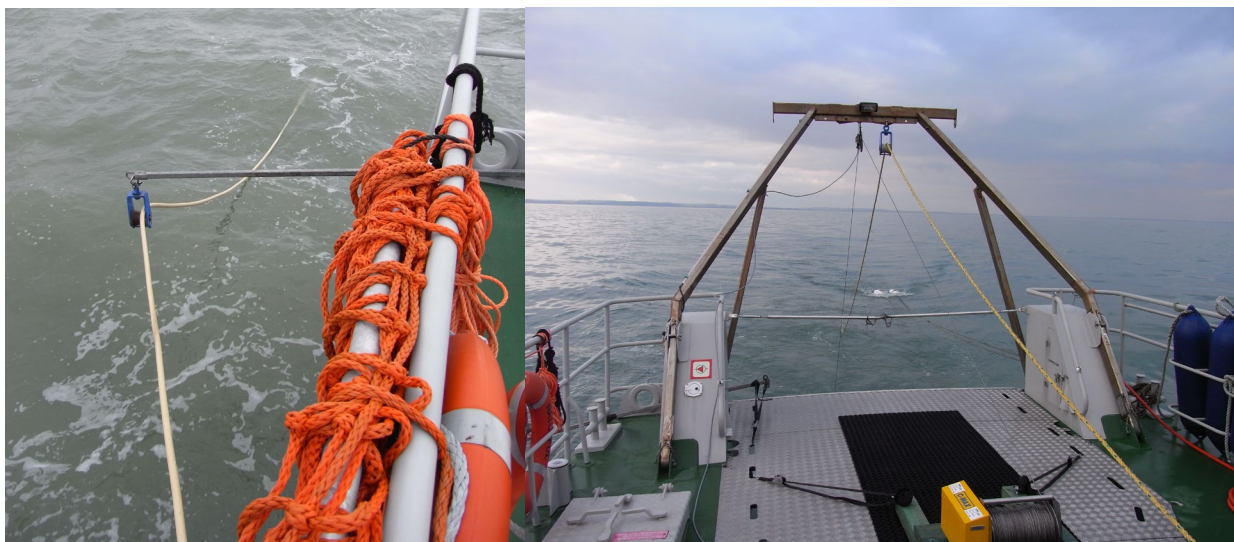
Figure 5 Left: BGS boom and hydrophone. Right: SSS counting pulley and STB block on A frame. SSS winch on deck.
