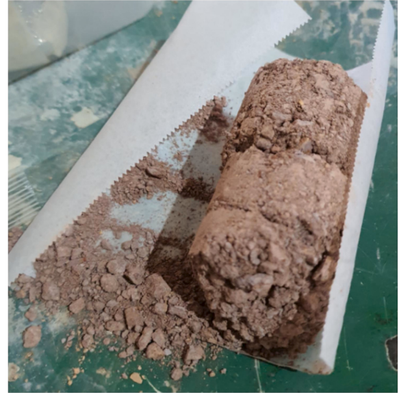
Fig. 5. Sample SC after curing for 28 days before conducting the UCS test. This sample was not treated with BVG liquid and was used as a control.
