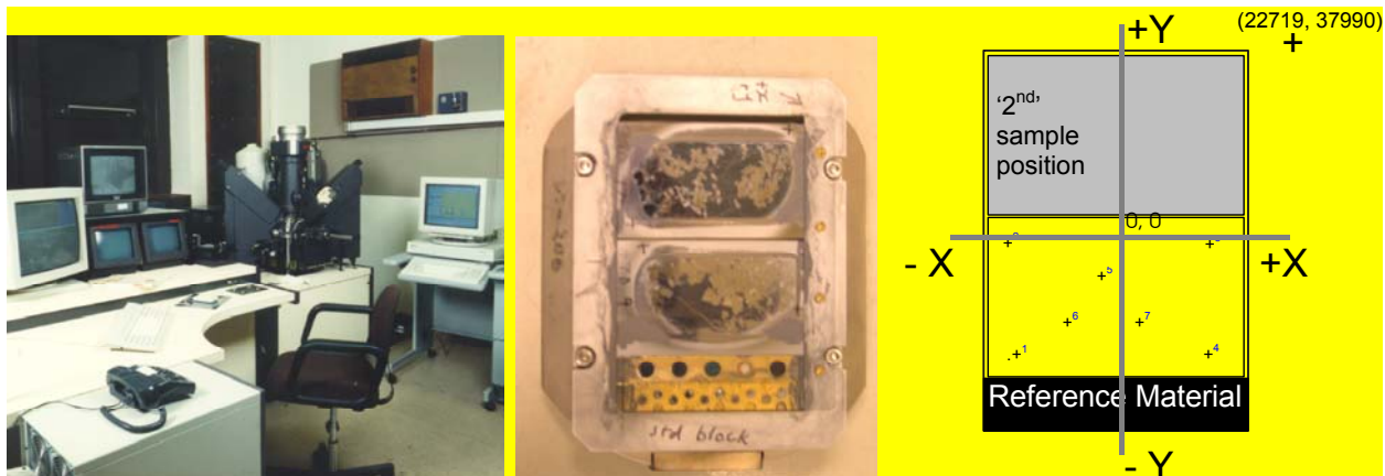
Figure 3. Position of the test sample holder within a Cameca sample holder, and relative directions of X- and Y-axes of the EPMA spatial referencing system.
