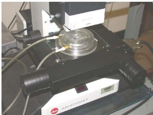
Plate 5 Digital X-Y stage attached to the light microscope used as part of the LA-ICP-MS instrument. This stage reads to a precision of 1 micron, and is under computer control such that the stage can be driven to the co-ordinates of points of interest. However, the sample cell (clear Perspex) offers relatively poor control on the orthogonality and positioning of the sample.
