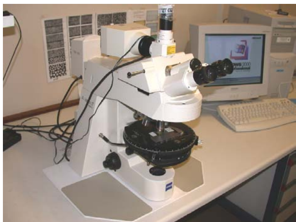
Plate 3 Simple, manual, X-Y sample holder attached to the rotating stage of a polarising microscope. The graticules on this type of sample holder can only be read to a precision of 100 microns.
