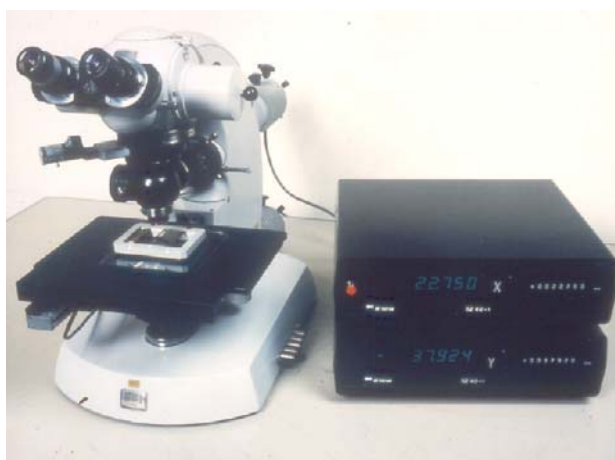
Plate 4 Digital X-Y stage attached to the conventional polarised light microscope used in association with the EPMA instrument. The sample is mounted in the sample block used in the EPMA instrument. This stage is highly orthogonal, reads to a precision of 1 micron and may have a user-defined “local” origin.
