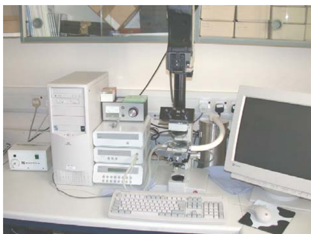
Plate 6 Digital X-Y stage attached to the light microscope used as part of the fluid inclusion microthermometric instrumentation (heating-freezing cell). This stage reads to a precision of 1 micron, and is under computer control such that the stage can be driven to the co-ordinates of points of interest. However, the sample material used in this cell represents sub-samples drilled from larger doubly polished wafers. The stage offers poor reproducibility of sample positioning, and the samples are typically too small for marking with the procedures outlined in the previous section.
