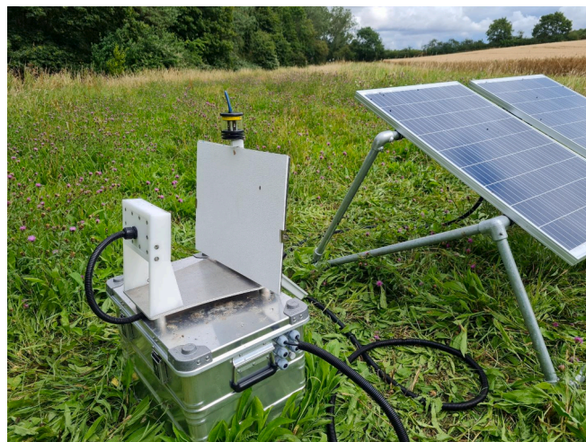
Fig. 1. The UKCEH AMI-system consists of solar panels (right), and a battery box (bottom), on top of which is a camera housing (left), a white landing board (right) – where insects land – and an attractant light (on top of the backboard). The electronics enclosure is mounted to the back of the backboard (not visible).
