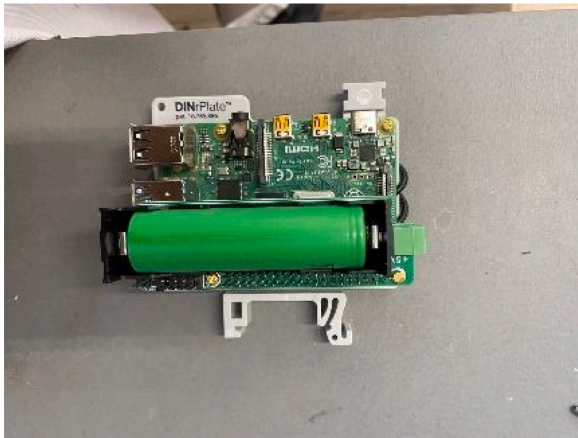
Fig. 9. Raspberry Pi and Watchdog mounted on top of DINrPlate.
