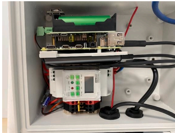
Fig. 10. All components attached to the DIN rail (wiring described in later steps).
