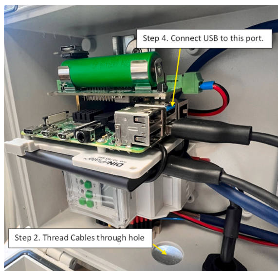
Fig. 12. Wiring the camera and lighting ring into the electronics enclosure, steps 2 and 4. See Fig. 17 for overview of electronics enclosure.
