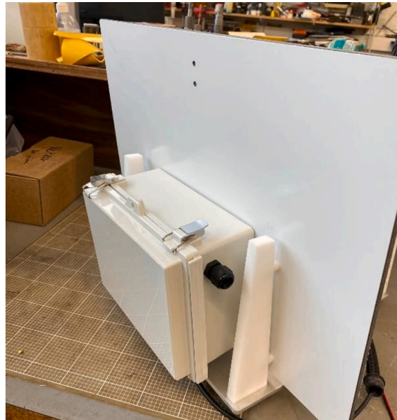
Fig. 18. Back board attached to the electronics enclosure and uprights.
