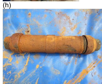
Figure 1 Observations of corrosion of handpump components made during the Hidden Crisis project in Ethiopia and Uganda. All photographs are of India Mark handpump components. (a) to (e) Corroded rod sections; (f) and (g) corroded rising main sections; (h) corroded cylinder. BGS © UKRI 2026.
