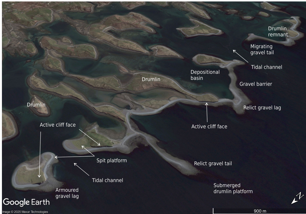
Fig. 2. The actively retreating drumlin coast and archipelago in Clew Bay, Ireland. Drumlin sediments from multiple point sources are reworked by waves and longshore drift into prograding, cusped spits, forming often gravel barriers that link drumlin islands. These barriers allow the development of depositional/lagoon environments connected by tidal channels. Many of the drumlin islands are linked, either by flanking barriers or gravel tombolos/tails. The progressive erosion of drumlin islands over time eventually leads to a flattened irregular platform with relict gravel tails or ridges. Maxar Technologies image dated 4/5/2007 courtesy of Google Earth.
