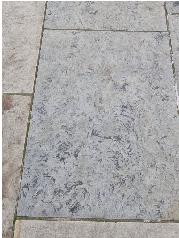
Above: Image showing a typical slab of the Whitworth Sandstone observed at Locality 9, when dry. The base colour of the stone, conspicuous dark cross laminae (creating a striking swirling patternation on the exposed surfaces) and limited development of Liesegang banding are all consistent with Whitworth Sandstone . Slabs of this stone appear to dry rapidly once wet.
