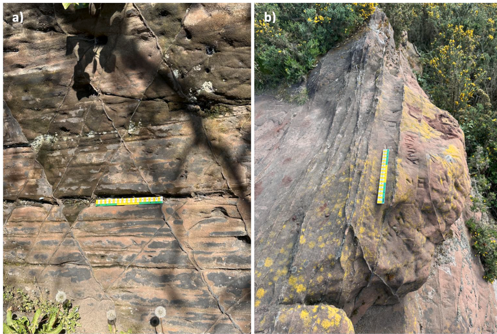
Fig. 1. a) Conjugate (diamond-shaped) deformation bands in a vertical cutting at Grange Hill, Wirral, NW England and b) a cluster of braided deformation bands on a horizontal surface of an outcrop at Thurstaston Common, Wirral, NW England. 30 cm ruler in each image for scale.
