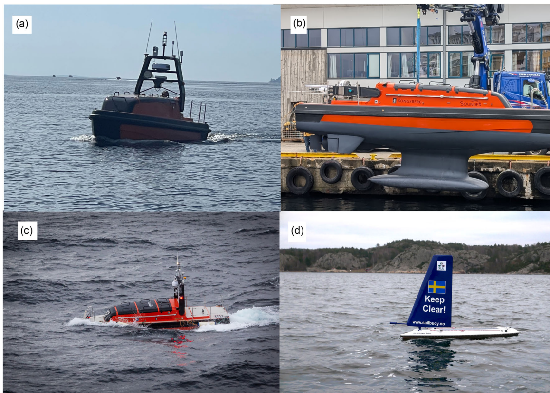
Figure 9. Examples of uncrewed vehicles used to collect data. USV Sounder from Kongsberg Maritime AS, (a) Brage Photo by Helge Sagen (IMR), (b) Photo by Caspar Christie (IMR), (c) Frigg Photo by Geir Persersen (IMR), (d) A sail drone with an echosounder, used by SLU Aqua, Sweden. Photo: Jonas Hentati Sundberg.
