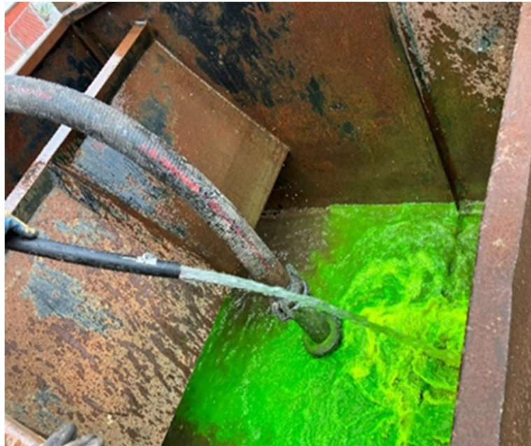
Figure 10 Sodium Fluorescein being added to the active tank system.
