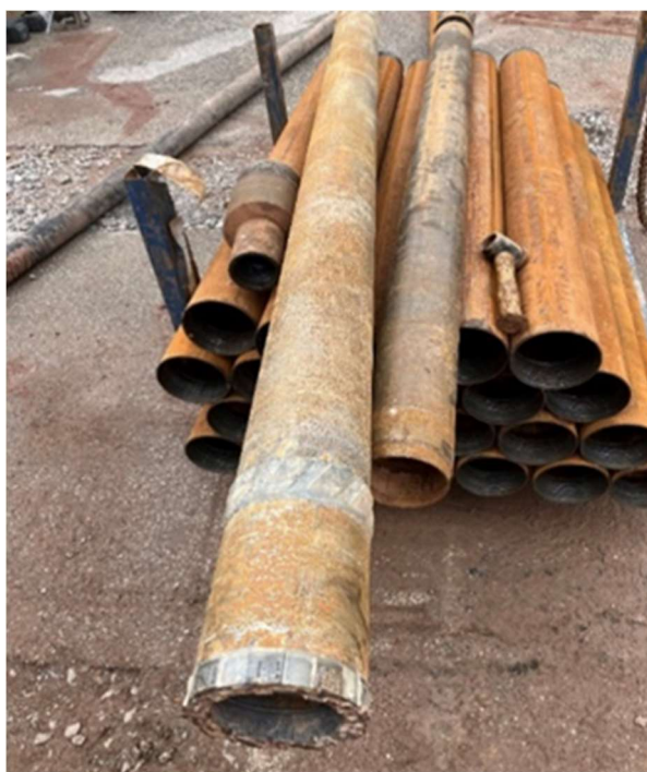
Figure 80 Image of the 146 mm Geobore coring assembly and rods
