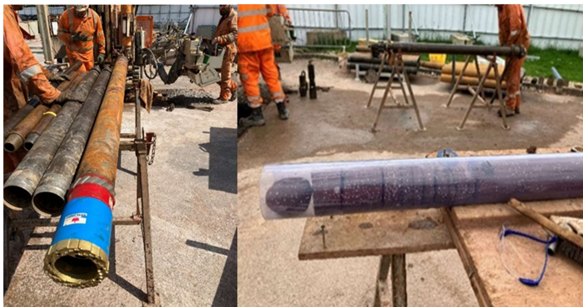
Figure 121 Lefthand image shows the 152 mm Geobore assembly, righthand image shows the fracture sandstone at circa 63.0 m.
