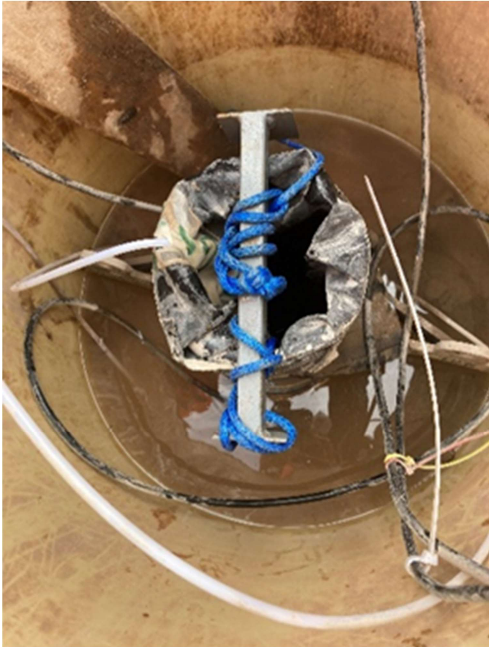
Figure 117 FLUTe liner deployment into TH0404
