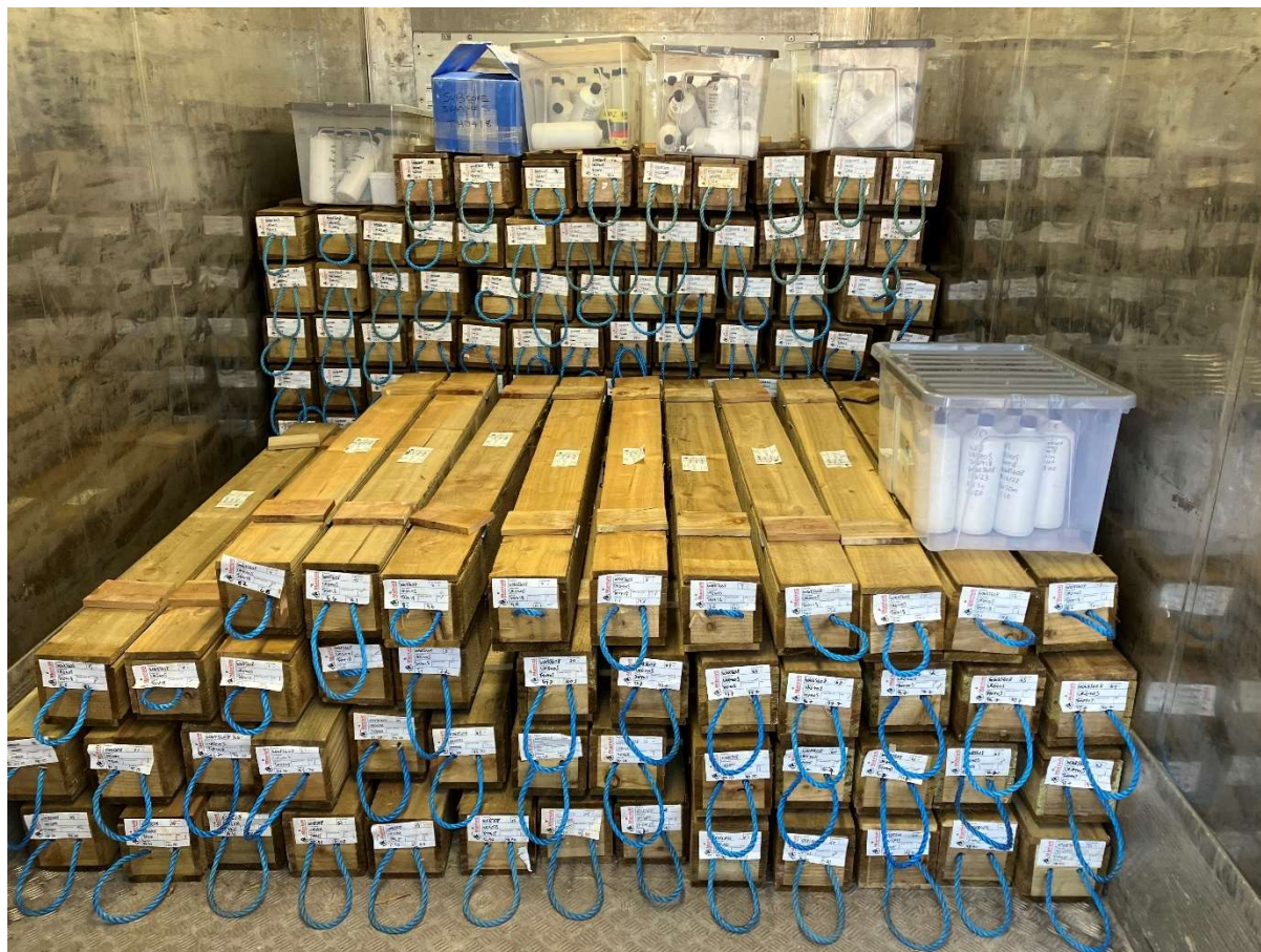
Figure 91 Recovered core and fluid samples from TH0407 in the cold store onsite
