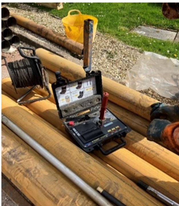
Figure 127 E-Totoc survey being taken
