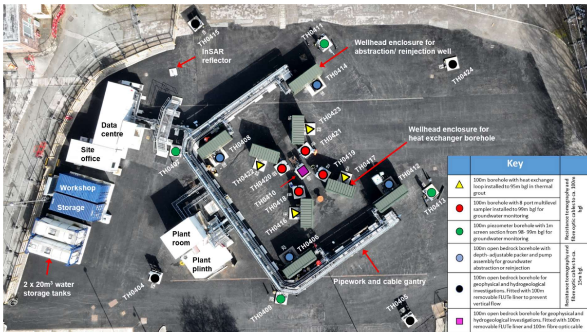
Figure 3 Aerial photo of the Cheshire site with the borehole array identifiers overlaid
