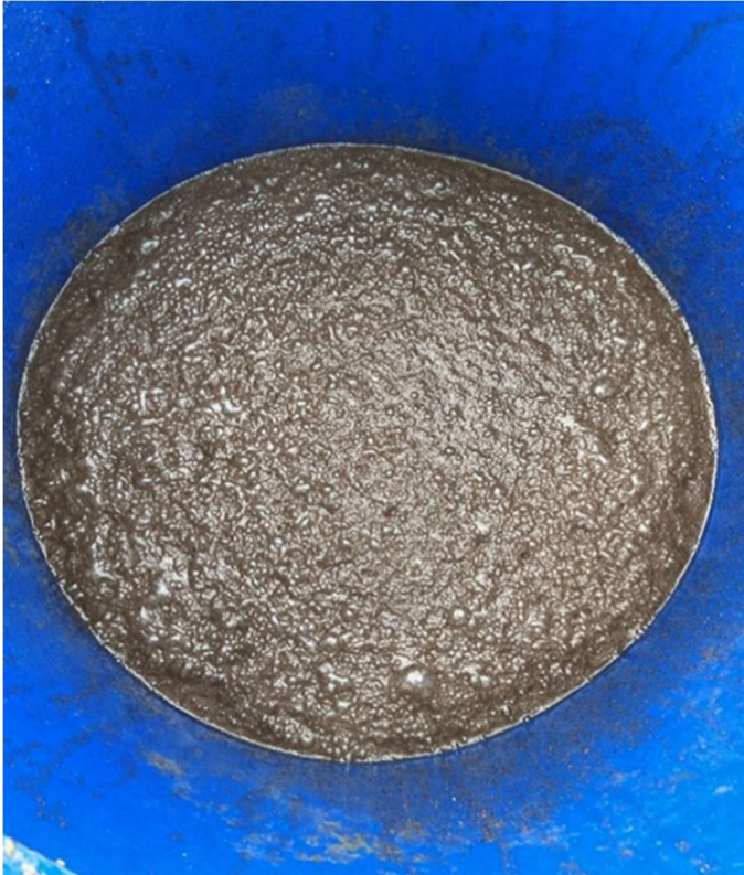
Figure 51 A 100 L 40 ppb LCM pill prepared ready to be pumped.
