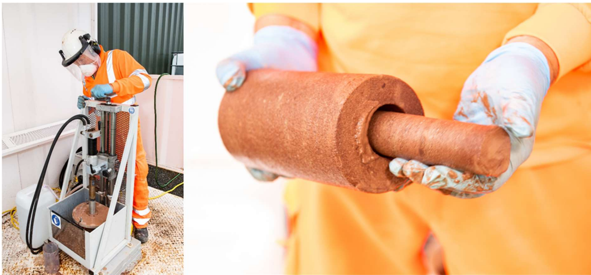
Figure 7 Sub- coring drill press and example sub-core
