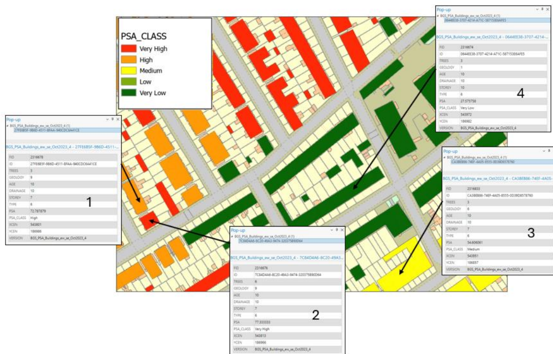
Figure 3 The BGS Property Subsidence Assessment dataset at building level, OS Open Map Local buildings are coloured according to the hazard class. Insets show the attribute values for 4 examples where the hazard score varies. Background is OS MasterMap for reference. Contains Ordnance Survey data © Crown Copyright and database rights 2024. OS AC0000824781. Contains National Statistics data © Crown copyright and database right 2024. Contains information sourced from Bluesky International Limited.
