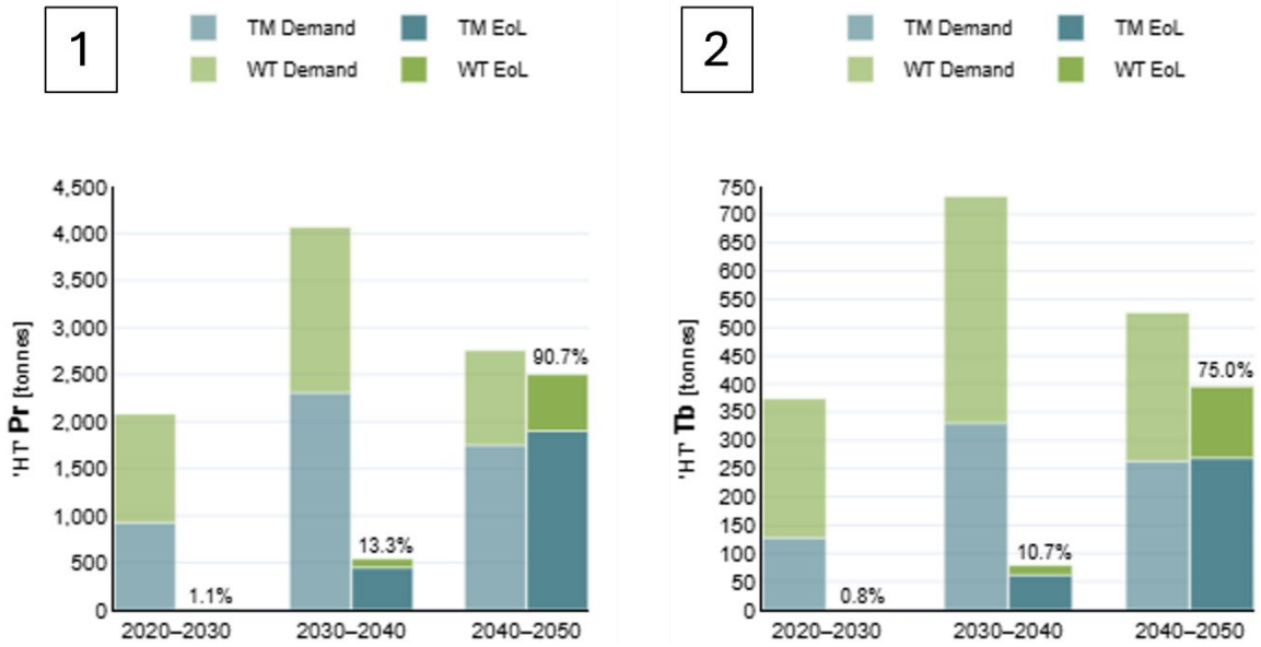
Cumulative demand and EoL quantities under the HT pathway for (1) Pr; (2) Tb in traction motors and wind turbines for the decades 2020 to 2030, 2030 to 2040 and 2040 to 2050. The unit is tonnes. BGS © UKRI 2026.
