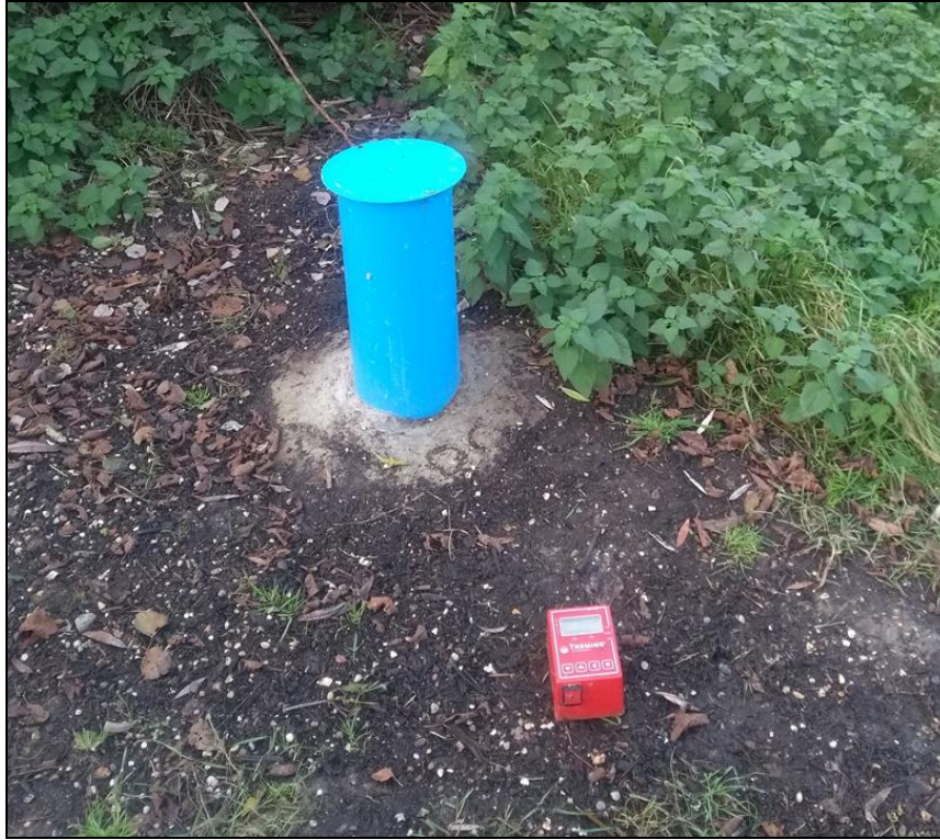
Figure 12. Tromino passive seismic instrument in operation next to a water observation borehole.
