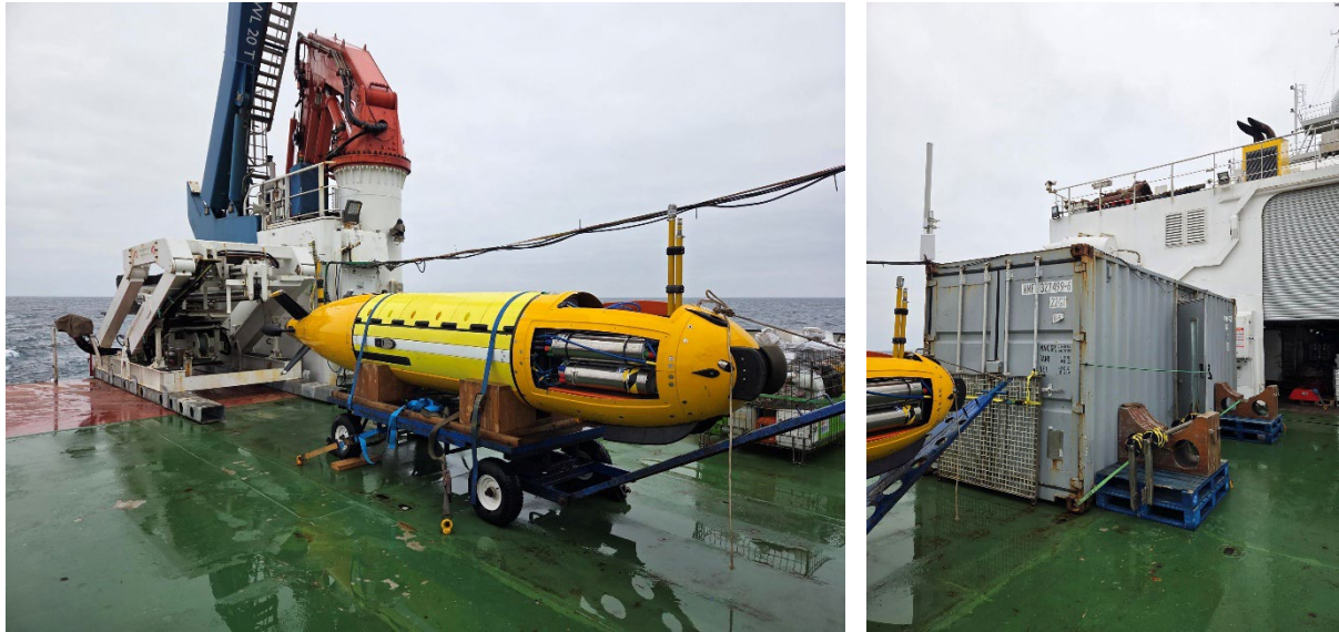
Fig. 6.7. Autosub 5 on its trolley after the last recovery, with the LARS already taken down to its storage configuration, on the afternoon of the second last day of the cruise.
