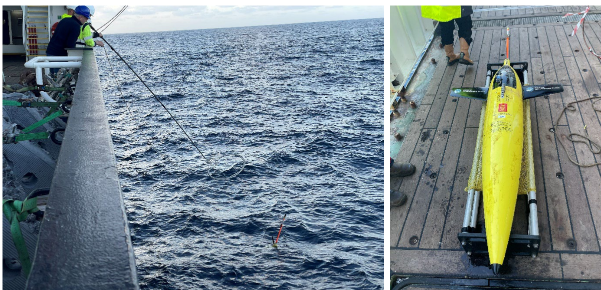
Fig. 6.29 Seaglider recovery using pole with lasso loop (left); Seaglider on board (right)
