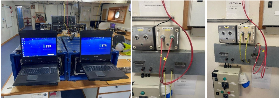
Fig. 6.24. Lab set-up: SeaSpyder topside station in the main lab (left). LEMO connectors (middle). LEMO connectors with earthing procedure (right)
