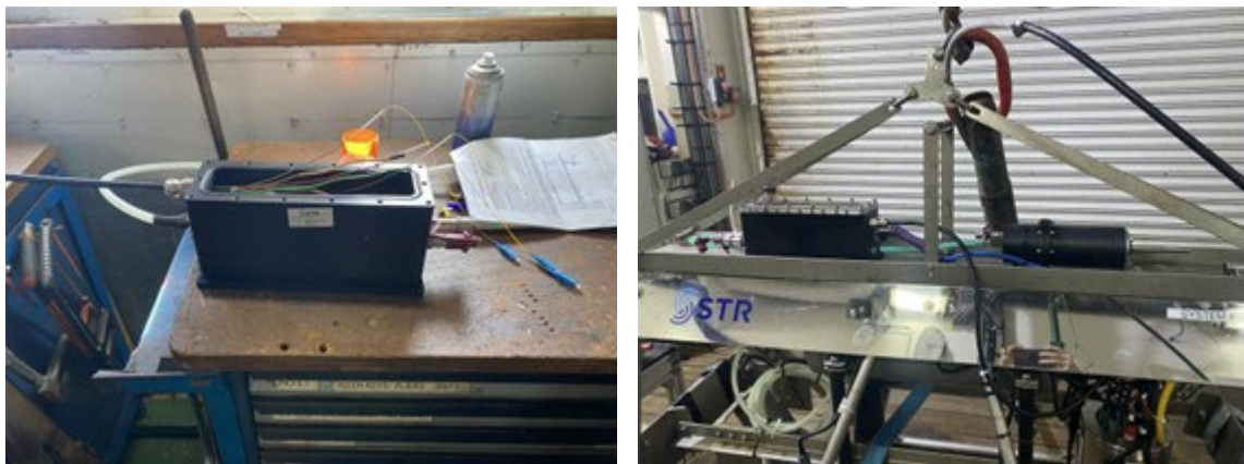
Fig. 6.23. Connection of the SeaSpyder to the ship's winch system: Deep tow winch termination showing fusion spliced fibre optic tails and STR SeaSpyder junction box (left). Mounted silicon oil filled junction box with oil filled pressure compensator on the SeaSpyder (right).
