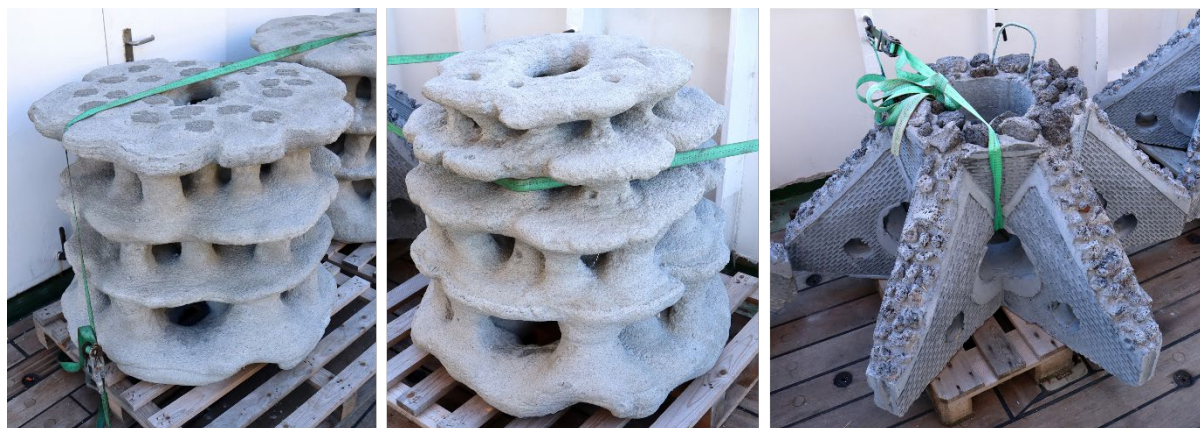
Fig. 7.28 Ecoreef models. Left and middle are the D-shape “wedding cake” type, AG900-3-REDRESS and AG800-5 , respectively, and right shows “star” type of the Life Lophelia project.
