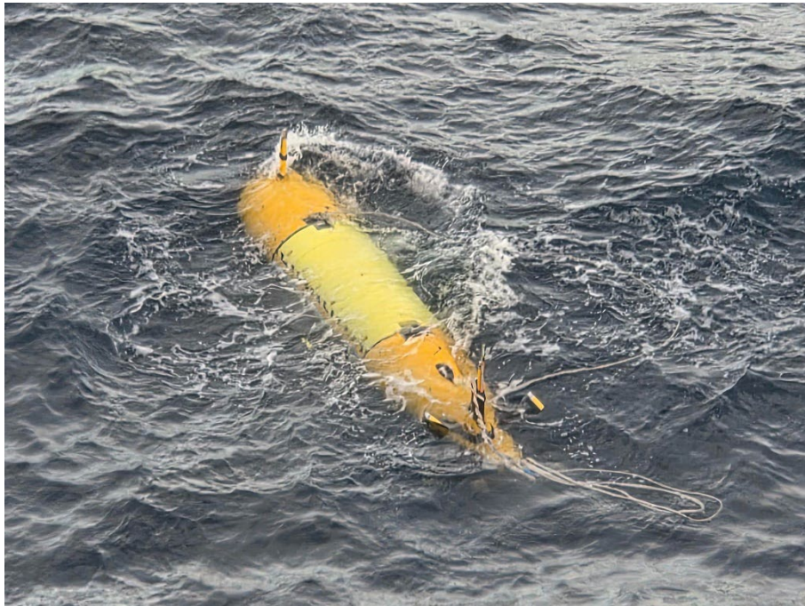
Fig. 6.13. Autosub 5 with its forward recovery line wrapped around the aft antenna mast.
