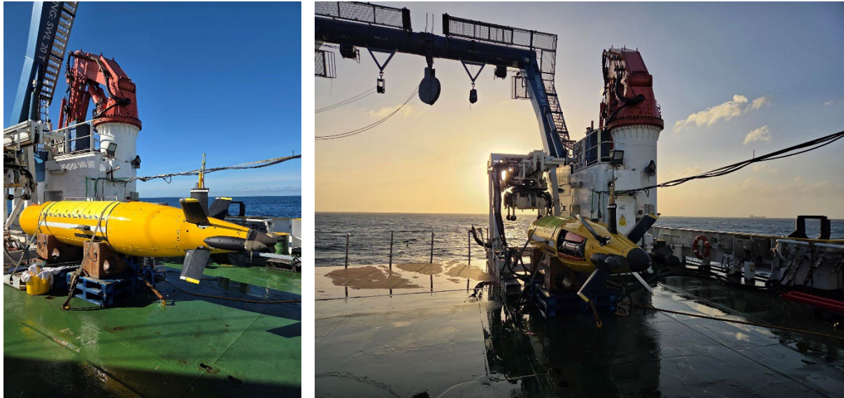
Fig. 6.5. Autosub 5 on the aft deck during non-operational times. The LARS is stowed away so that the top of AUV can be accessed with ease.
