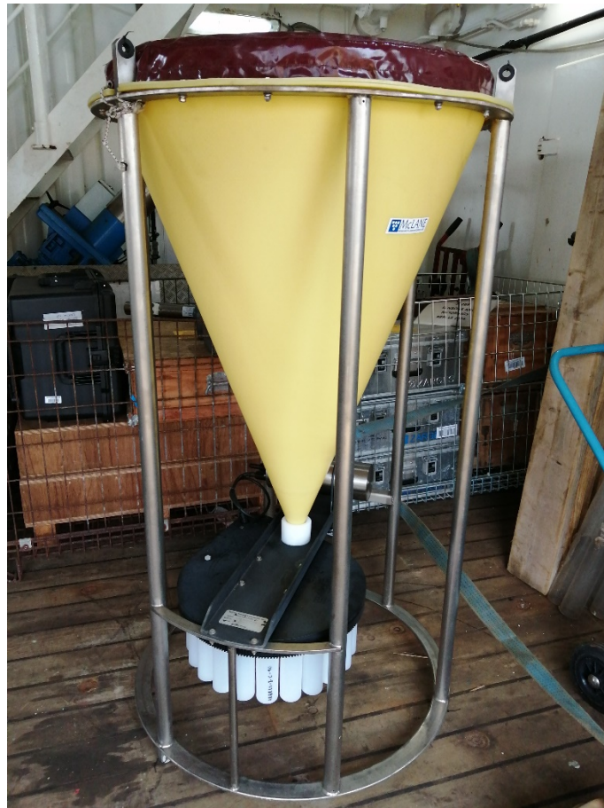
Figure 24: One of the three sediment traps prepared for ReBELS loaded on RRS James Cook.
