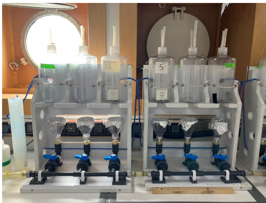
Figure 9: Filtering rig in the wet lab of the RRS James Cook that was used to filter for HPLC (not the samples from events 49, 50 and 53), POC, PIC and BSi.
