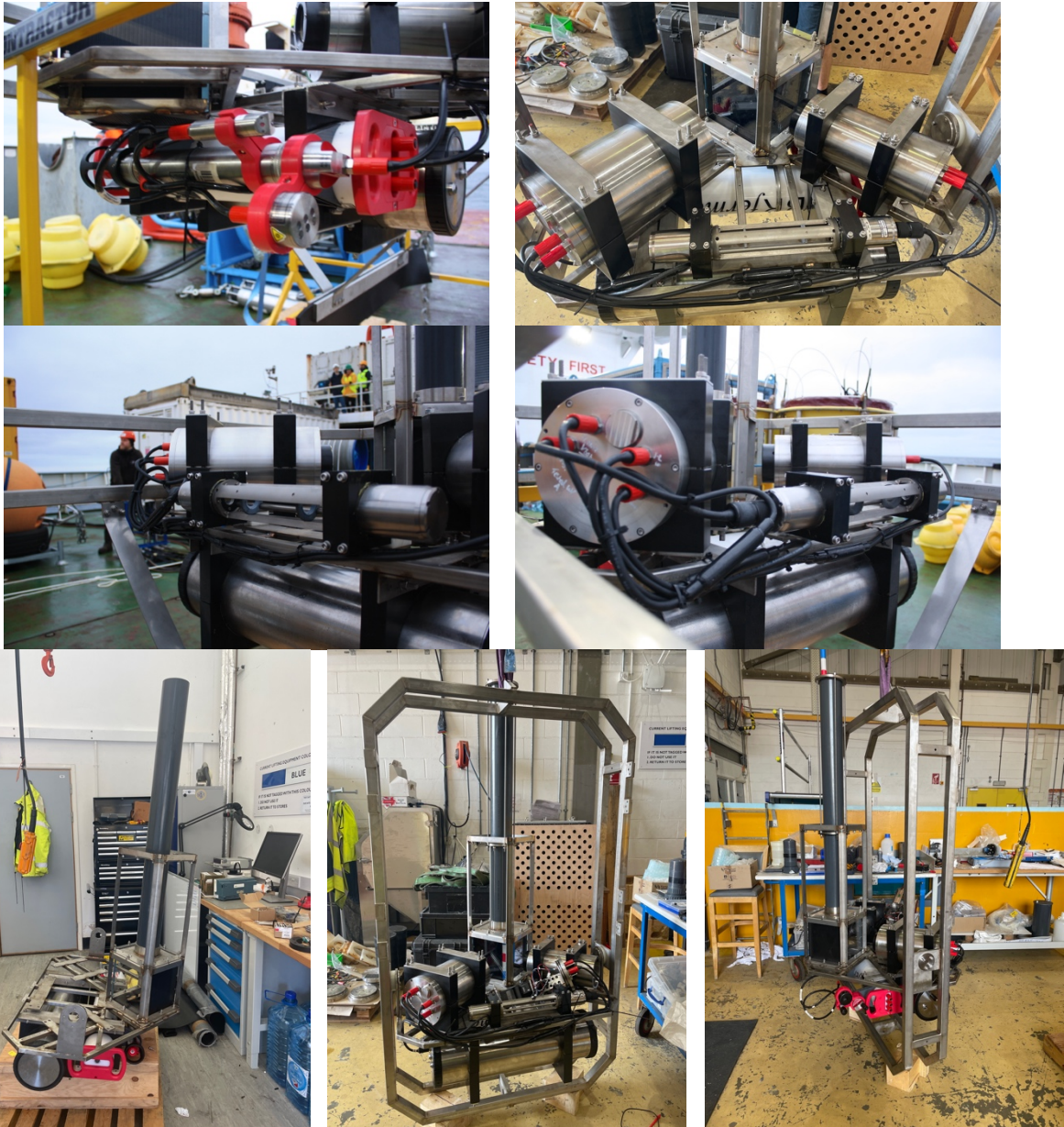
Figure 21: different views of the fluxCAM setup, including the RBR logger and batteries; top view of the camera and flash housings and transmissometer; and detail of the pivot table without the camera and flash housings, and front and side views of fully assembled system
