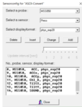
Figure 35: Window on the SSDA_228 software with the selection of drop-down options necessary to process the data.
