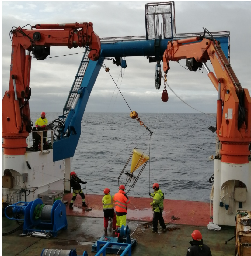
Figure 26: Deployment of one of the three sediment traps on 21/08/2024 as part of the ReBELS mooring.
