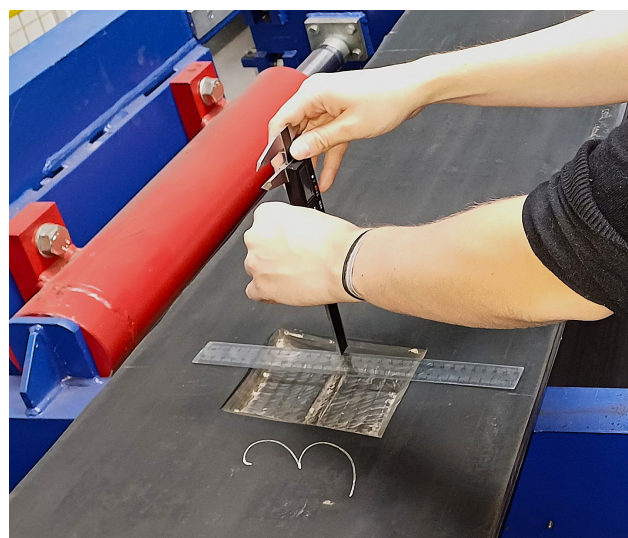
Figure 8. Hand measurement of defect size using a ruler and caliper.
