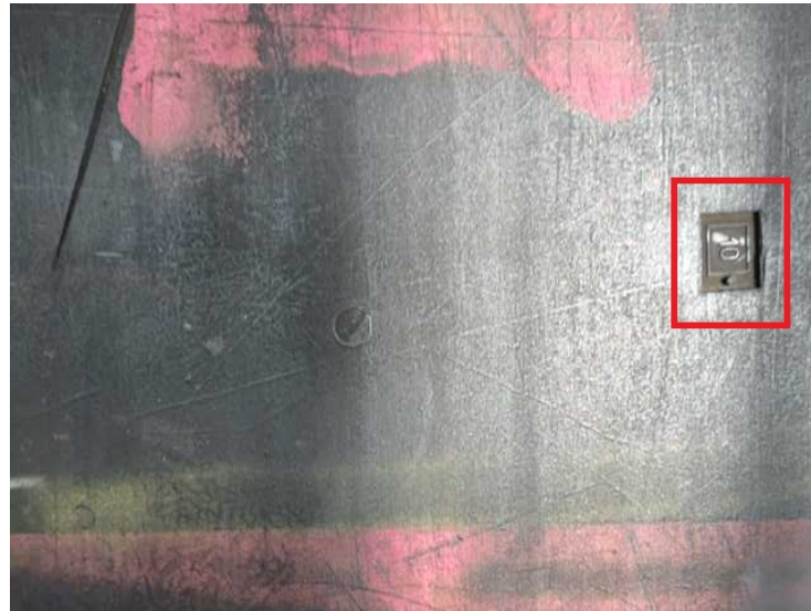
(a) A belt patch (red box) captured by RGB camera
