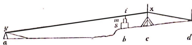
Figure 2. Schematic from CG05 of the tide gauge used at Sorgfjord in 1900. A wire “aixd” passes over a tripod at point “a” on floating ice approximately 80 m from the shore, and points “b”, “c” and “d” on land. A thinner wire extends vertically from “i” on the main wire through a container and is attached to a slide with a crayon that writes on a chart recorder “m”. As a result, variations in the level of the ice at “a” are reproduced on the chart recorder “m” scaled by 17.22 to 1. (Source: Carlheim-Gyllensköld, 1905)
