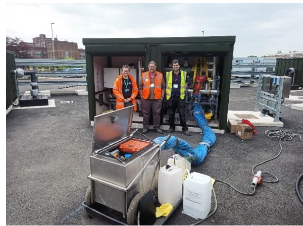
Figure 4: Photo showing typical test set up using the Rock Geotechnical TRT rig. Taken on 20 May 2024 at well TH0416 by Mike Spence. BGS © UKRI
