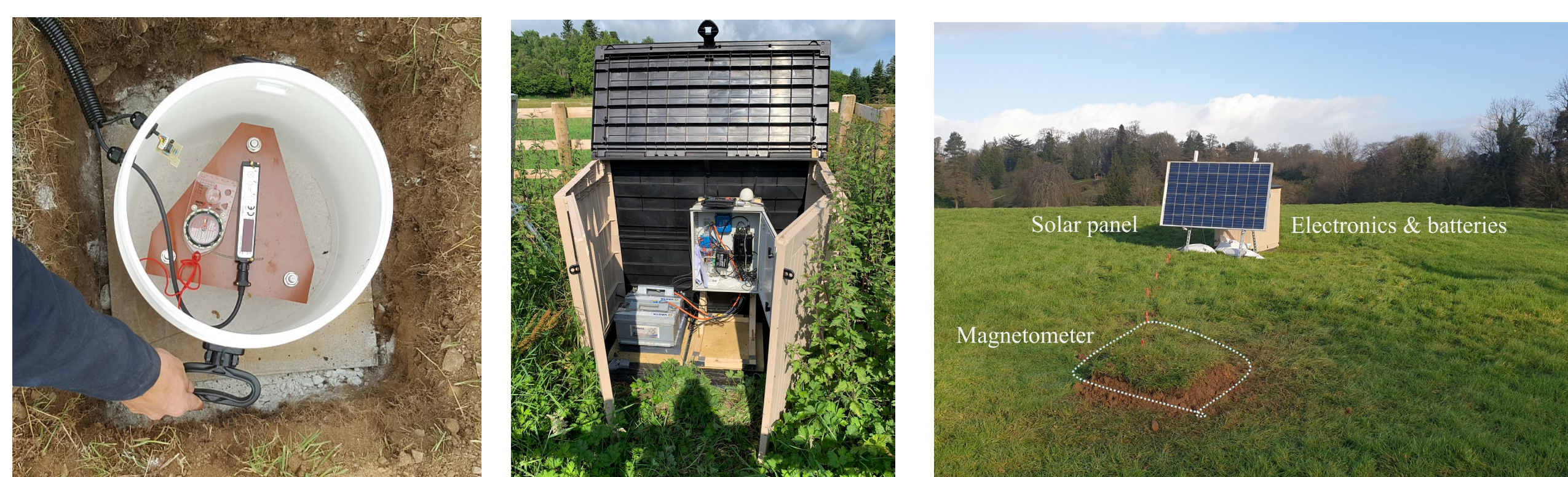
Figure 5 Left: The magnetometer within a barrel, in the pit. Middle: Plastic shed containing the electronics and batteries. Right: Photo of the complete installation at FLO
