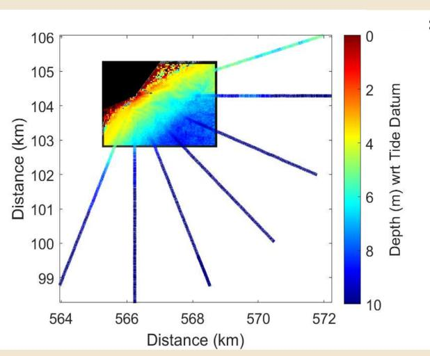
X-Band radar bathymetry overlaid with SBES survey data
