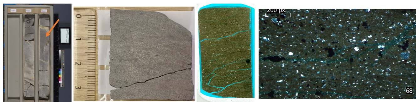
FIGURE 8 | Core, thin-section scan and thin-section micrographs comparing the (micro)texture of a soft and hard mudstone. While both display disrupted fabrics, these fabrics are most likely associated with bioturbation. No obvious deformation fabrics are observed in the hard mudstone, although we may be looking for rather cryptic fabrics associated with deformation of soft mudstone. Top: BGS Sample number SSK144262. Bottom: BGS Sample number SSK144262.
