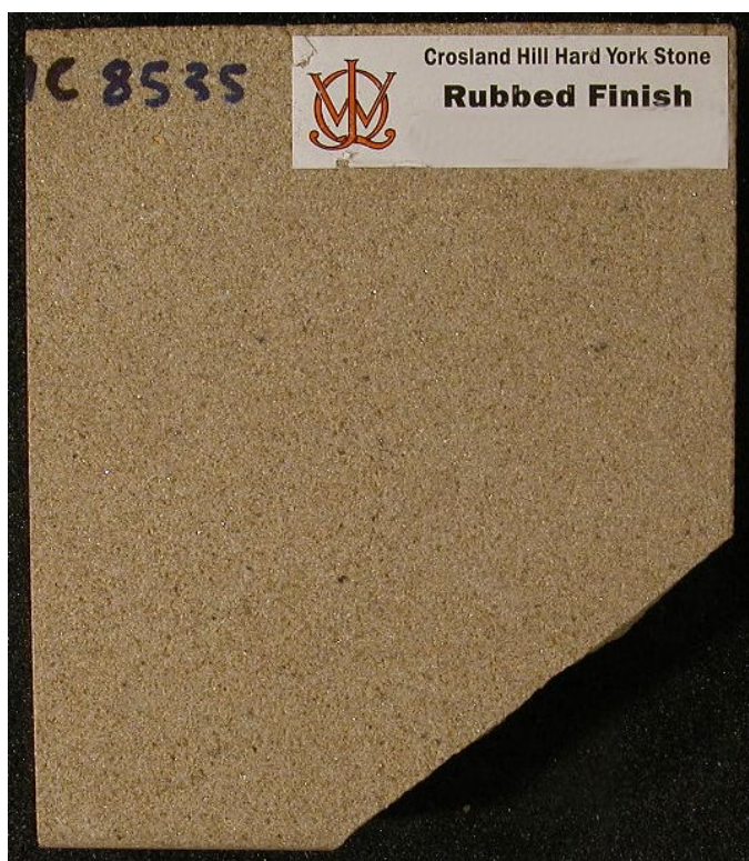
Photo 74. Sample of Crossland Hill York Stone, typical of many Yorkshire sandstones currently used for paving, showing typical buff colour and uniform appearance.
