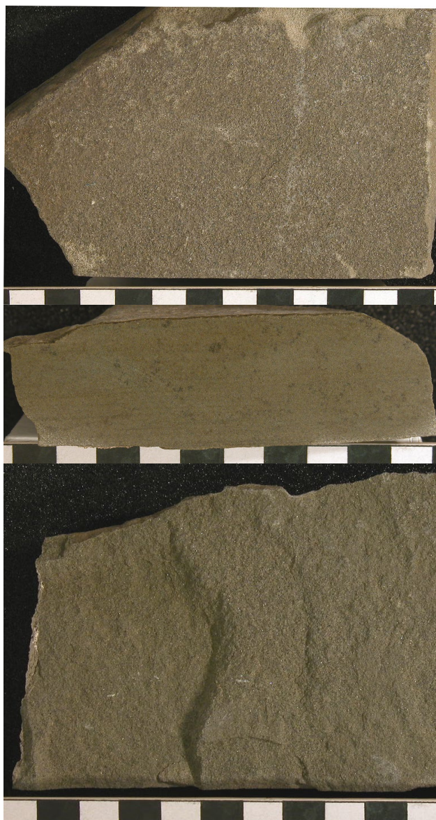
Photo 68. Samples of Angus sandstone paving from the Edinburgh New Town. Top and centre images are from General Register House (samples ED10194 & ED10189), showing a natural paving surface (top) and freshly broken surface (centre). Bottom image is from St Stephen's Place (sample ED10145) showing cut section through paving slab illustrating the bedded texture with faint parallel laminae. These samples are typical of 'Angus type' flagstone with a very fine grained compact texture, with grey green colour. Scale divisions are cm.
