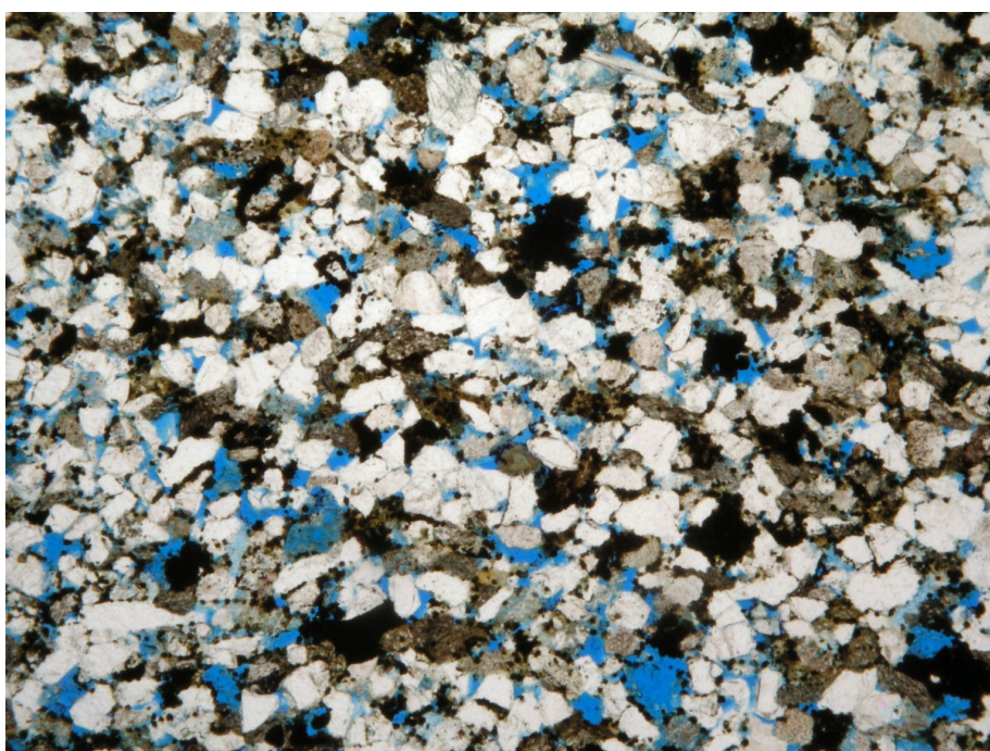
Photo 75. Microscopic thin section image of sample of pavement from Register House (Top image) and sandstone from Woodkirk quarry, near Leeds (Bottom image), both showing uniform fine to medium grainsize with moderate porosity and abundant brown iron-bearing minerals. Image c.3 mm across, plane polarised light; porosity highlighted by blue dye resin.
