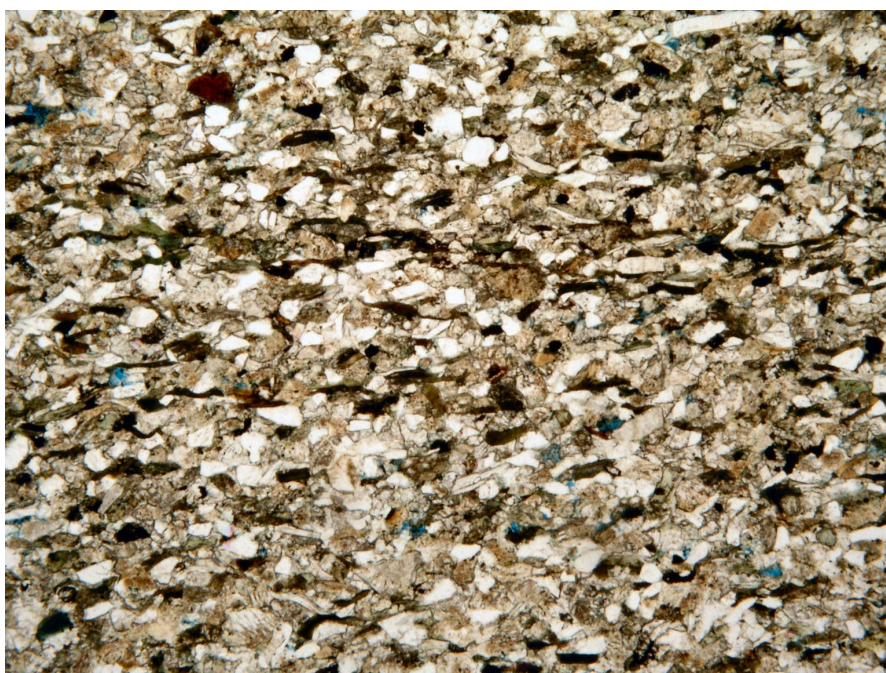
Photo 69. Microscopic thin section image of sample of pavement from Register House (Top image) and sandstone from Carmyllie quarry in Angus (Bottom image), both showing fine grained compact texture with little porosity, with a complex mineral composition seen by the abundance of dark and brown iron-bearing grains. Image c.3 mm across, plane polarised light; porosity highlighted by blue dye resin.
