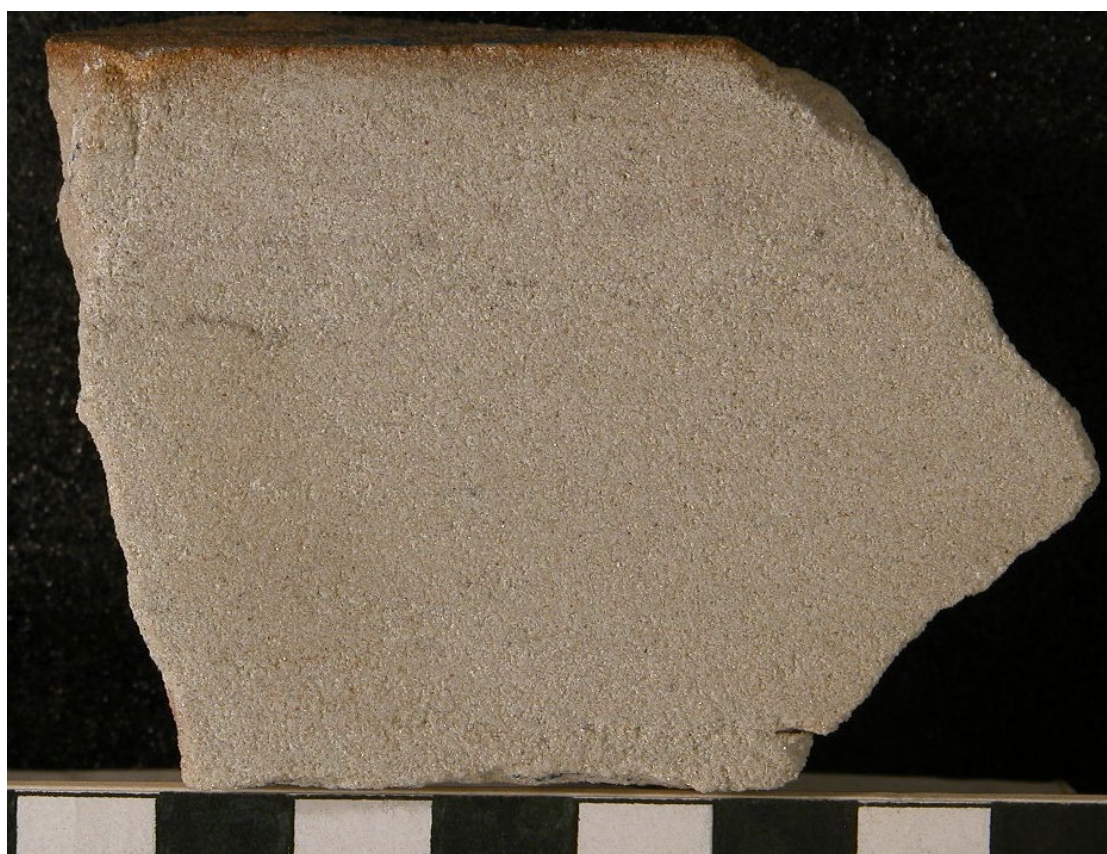
Photo 64. Cut section through sample of paving from General Register House showing typical ‘Craigleith type’ characteristics with very pale quartz-rich sandstone with medium grainsize and uniform texture. Note the top weathered surface with an orange-brown patina, distinctive of this type of stone, formed by weathering of microscopic iron oxide grains throughout the stone. BGS sample ED10186. Scale divisions are cm.
