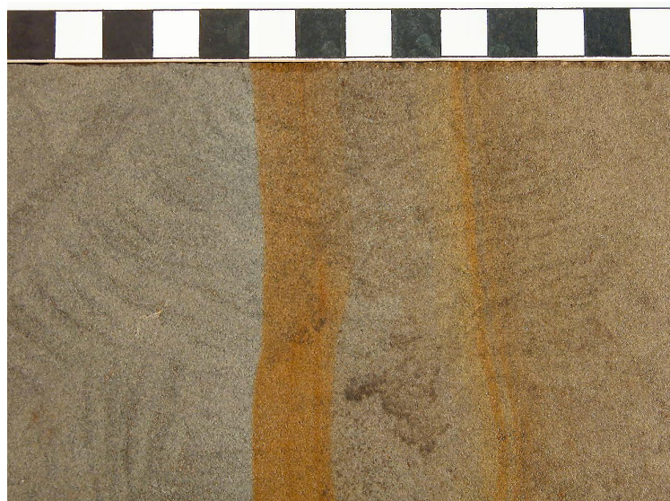
Photo 78. Sample of Scout Moor sandstone showing sawn top surface with variable colour from grey to orange-brown, and ‘contour-effect’ texture caused by the presence of fine ripple bedding laminae. These characteristics are similar to those of Hailes type sandstone. Scale divisions are centimetres.
