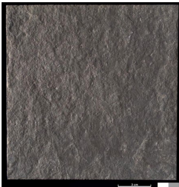
Photo 70. Sample of Caithness flagstone from Spittal quarry near Halkirk, showing typical dark colour and fine grained texture, giving characteristic distinctive appearance. Natural riven surface.
