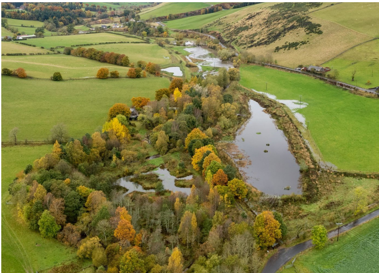
Kidston Mill flood pond under flood conditions Nov 2021. Note also flooded new meanders upstream at Nether Kidston
