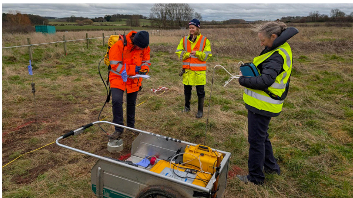
Figure 23 BGS mobile field soil gas facility like that used to take gas and flux measurements during this incident. BGS © UKRI.
