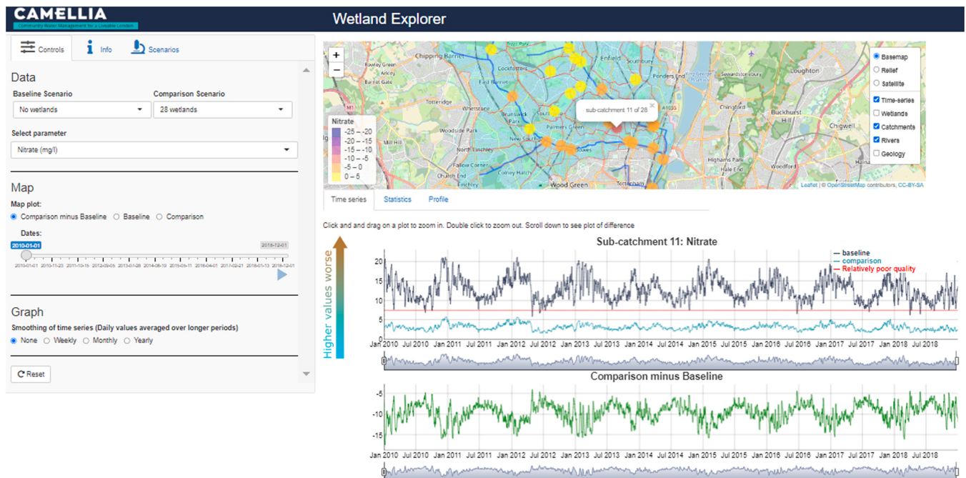
Fig. 2. © 2025 CAMELLIA. The Wetland Explorer web interface. The controls through which the user manipulates the display of information (scenarios and parameters) are on the left-hand side. The map with clickable dots representing the sub-catchments is on top right. Below that is the graph that display time series with an arrow indicating the physical meaning of the values displayed to the immediate left there are also options for the graph to show statistics or profile for the selected sub-catchment. The actual Wetland Explorer, with interactive features and animations can be accessed at: Removed for anonymization .
