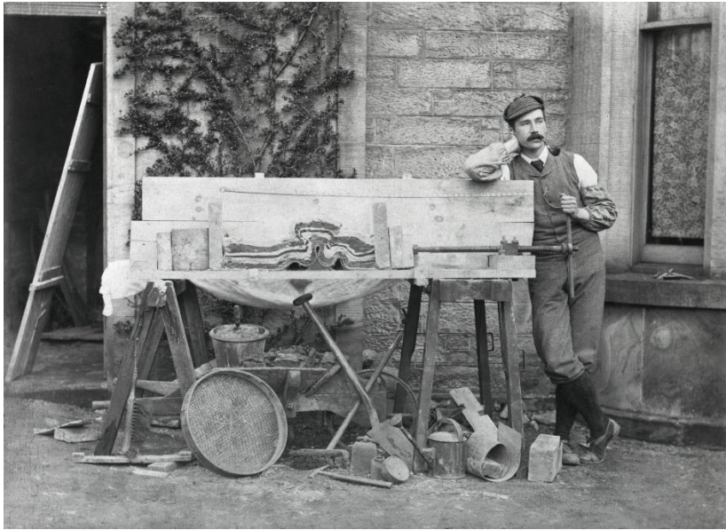
Figure 2. Cadell in 1885 experimenting with his 'squeeze box' to model fold and thrust development. British Geological Survey image P240116 © UKRI.
