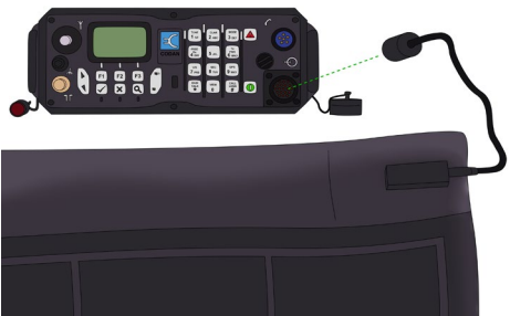
Figure 49 – Connecting solar panel to charge battery
