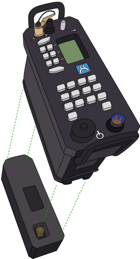
Figure 47 – Connecting battery to radio
