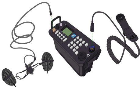
Figure 46 – Connecting co-ax and handset
