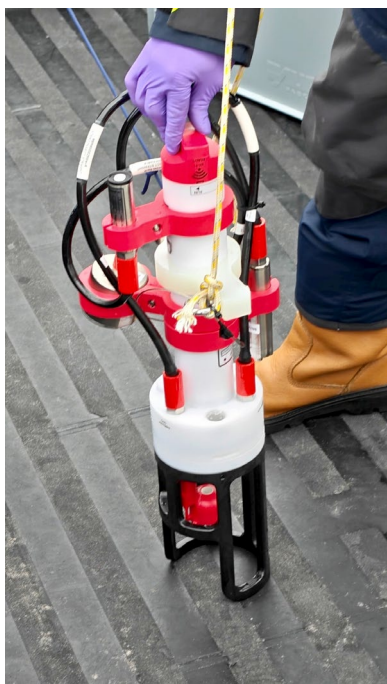
RBR Maestro CTD, and the hand deployment of the CTD and Niskin bottle
