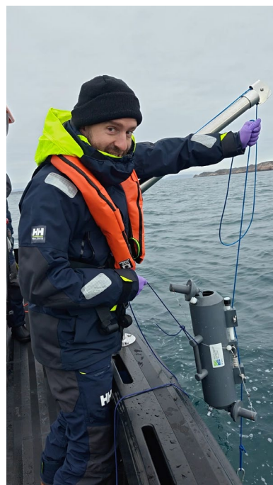
RBR Maestro CTD, and the hand deployment of the CTD and Niskin bottle
