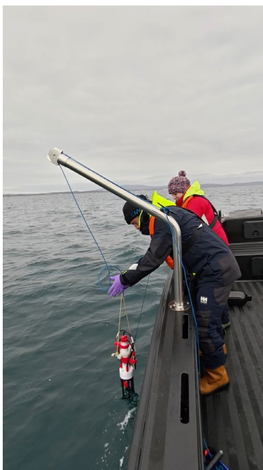
RBR Maestro CTD, and the hand deployment of the CTD and Niskin bottle
