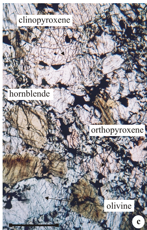
Plate 6. (a) and (b) Fine- to medium-grained metadunite containing anhedral crystals of talc (plane and crossed polarised light. Sample S22026). (c) and (d) Hornblende metaperidotite containing both clinopyroxene and orthopyroxene (plane and crossed polarised light. Sample S2934). Scale bar = 1 mm
