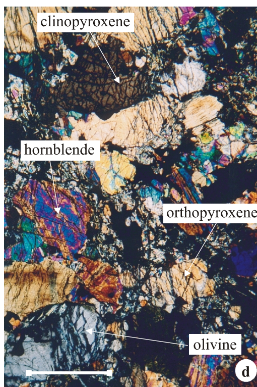
Plate 6. (a) and (b) Fine- to medium-grained metadunite containing anhedral crystals of talc (plane and crossed polarised light. Sample S22026). (c) and (d) Hornblende metaperidotite containing both clinopyroxene and orthopyroxene (plane and crossed polarised light. Sample S2934). Scale bar = 1 mm
