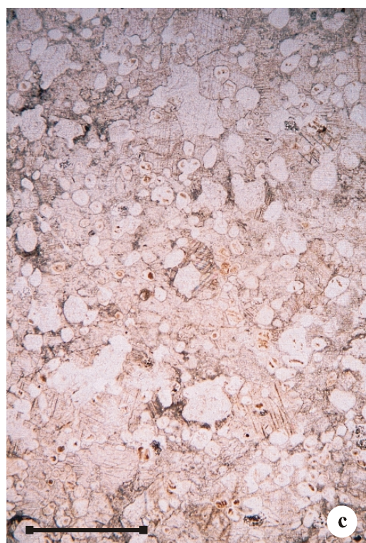
Plate 13. (a) and (b) Brucite marble (plane and crossed polarised light. Sample S9208). (c) and (d) Forsterite-brucite marble in which all the olivine has been replaced by serpentine (plane and crossed polarised light. Sample S9843). Scale bar = 1 mm
