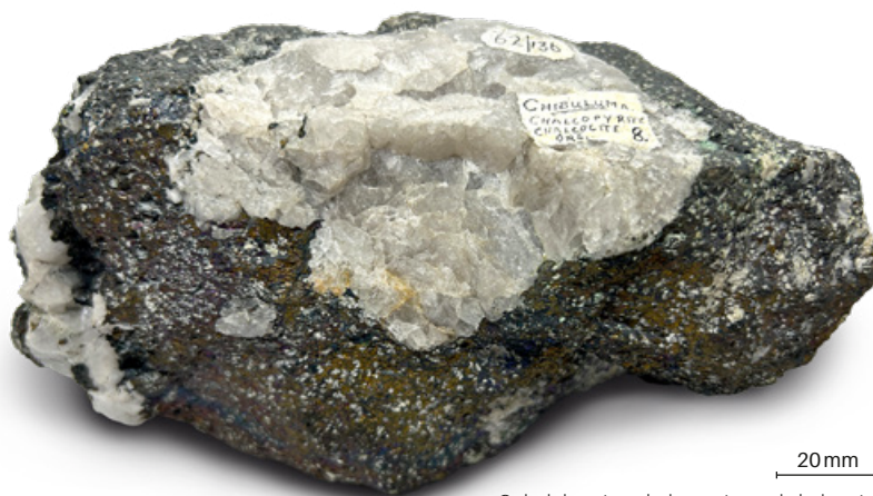
Cobalt-bearing chalcopyrite and chalcocite ore, Chibuluma, Copperbelt Province
