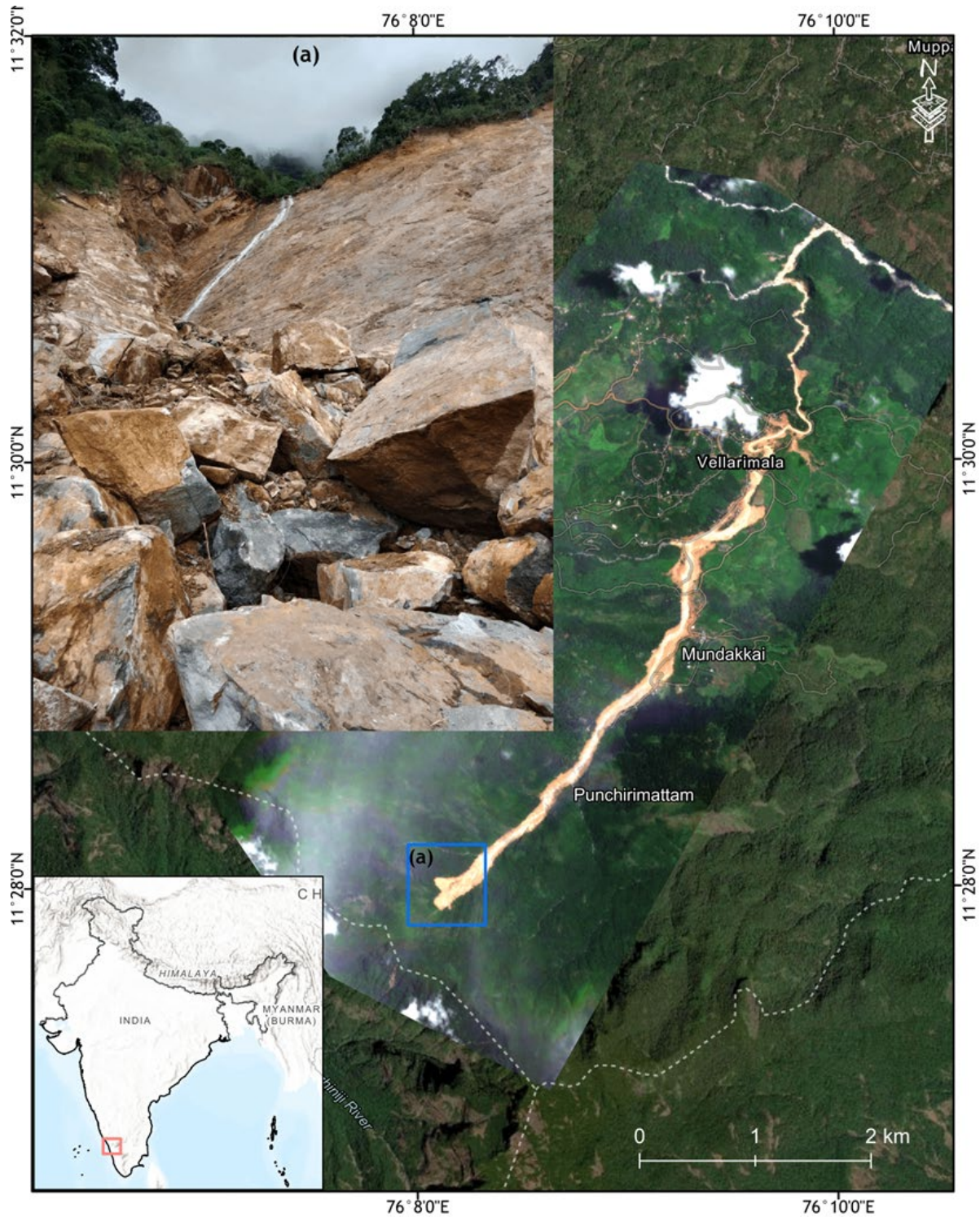
110 111 112 Figure 1. Map showing the location of Wayanad Landslide. (a) Landslide scarp area reveals 113 evidence of a planar rock slide. Large boulders remain below the crown, posing a potential risk 114 for future, especially during periods of heavy rainfall. 115 During the extreme rainfall event of 2020, a comparatively smaller landslide originated from the 116 same source region, and its runout length reached ~5 km downstream, but was mostly confined 117 within the riverbanks. The primary destruction from this 2024 July event is believed to have been
