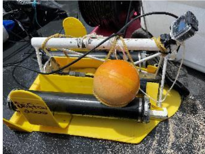
Figure 11. AIG Drifto 2000 with BGS GoPro 11 attached.
