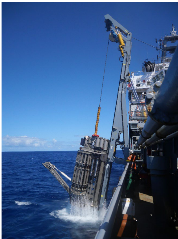
Figure 13 PROD5 being launched during IODP Exp. 389, Hawaii. Credit: M. Rydzy, ECORD-IODP.
