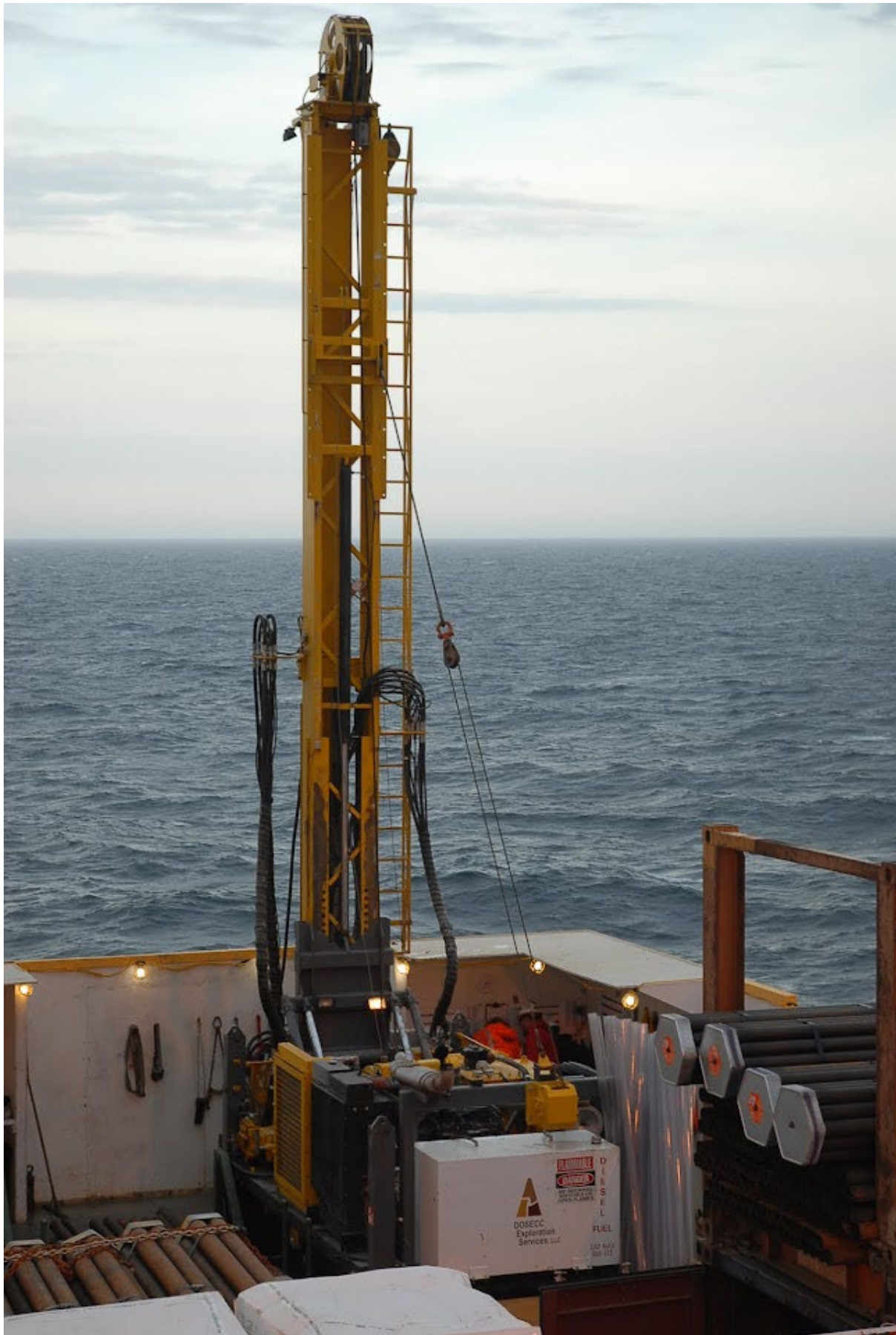
Figure 7 Atlas Copco CS4002 mining rig on IODP Exp. 313. Credit: Graham Tulloch, ECORD-IODP.
