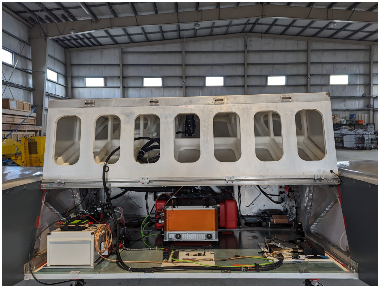
Figure 11. Gravity and magnetic floor. The grey box on the left is the power distribution. The orange box in the centre is the iMAR gravity system. The boxes on the right of the floor are the magnetometer system, including logger, fluxgate and inertial navigation system. The magnetometer sensor in the payload bay door is linked to the logger by the thick black cable. The cable in the lower left goes to the 28 V ground power supply used to maintain the iMAR system at temperature.
