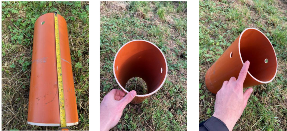
Fig. 4. PVC pipe with two custom-made holes at one end and bevelled opposite end.
