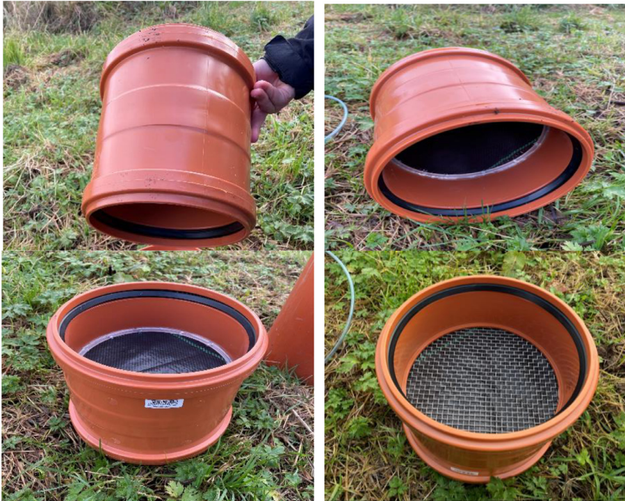
Fig. 5. PVC solvent welded double socket coupling with acrylic ring base, a woven weed control mesh and a geotextile membrane in the middle.
