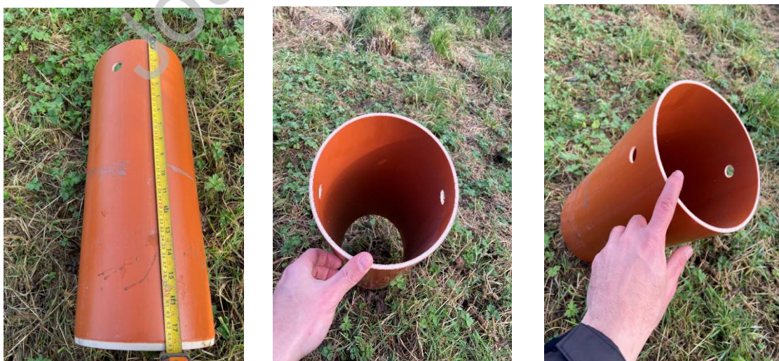
Fig. 4 PVC pipe with two custom-made holes at one end and bevelled opposite end.
