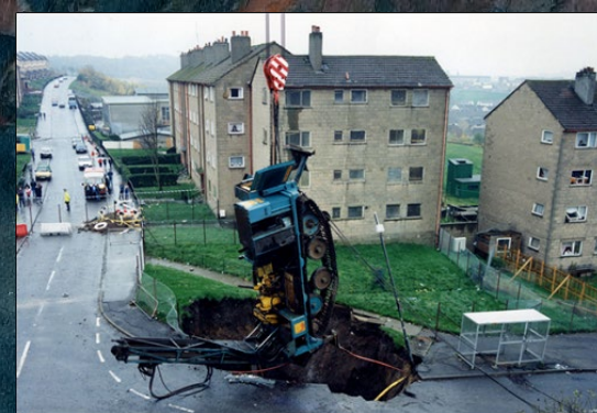
Drilling rig pulled from a collapsed mineshaft, Glasgow, Scotland. (Credit: BGS, UKRI)
