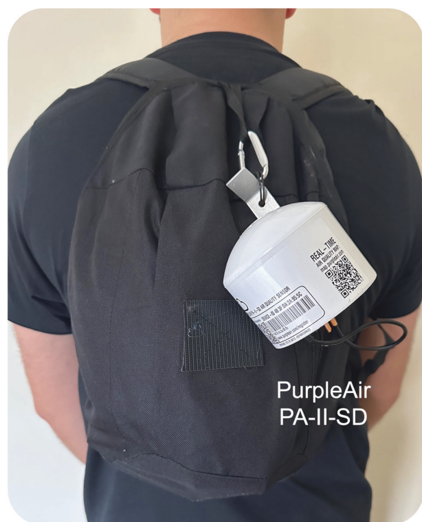
Fig. 2 PurpleAir attached to customised backpack and powered by battery pack (inside). The PurpleAir was secured in place with Velcro to minimise agitating fibre particles and to keep the sensor as close as feasibly possible to 'breathing zone' height. When stationary for long periods, the participant was permitted to remove the PurpleAir from the backpack and keep it close-by (as in McCarron et al. [26]).
