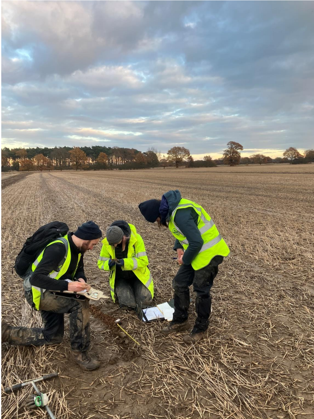
Figure 5. Litho-genetic mapping of glacial lake sediments in the Vale of York using surface morphology and a soil auger to capture shallow cores of sediments. © BGS 2024.
