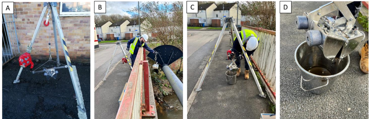
Figure 2: Images demonstrating safe use of the clam shell sediment grab sampler in the field from a height when bridge sampling from the central channel. Due to the weight of the full sampler on return, a tripod and winch may be necessary as demonstrated here. For lower height sampling a rope will suffice. A) shows the grab sampler and winch assembly, B) demonstrates adequate sampling location for bridge sampling the centre of the channel, C) the grab sampler is opened manually and D) the captured sediment is decanted into the cleaned steel bucket. As the grab sampler can capture both the solid sediment and some of the overlying water, it is allowed to settle before the majority of the supernatant is decanted and the sediment solids taken for sampling.
