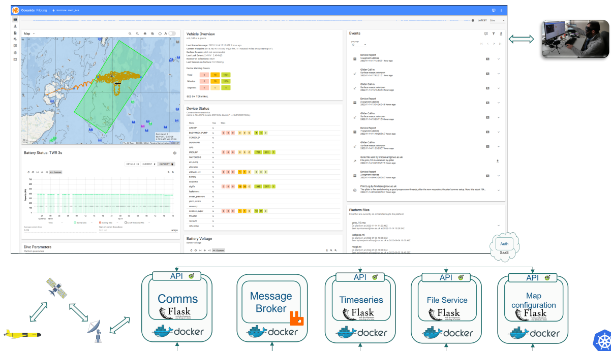
FIGURE 3. This is our piloting App, operating an ocean glider in the north sea. The robot calls using satellite communications to a base station. Our C2 system monitors the base station with a microservice managing incoming and outgoing communications. When an incoming communication arrives, the communication microservices tell the rest of the microservices using RabbitMQ, and each interested microservice accesses the information from the communication microservice using APIs. All the microservices use the same communication flow. Our frontend calls the different microservices APIs to show pilots the operational state and then sends operator instructions to the vehicles. In this figure, we are still showing our old authentication provider. The whole system is running on a Kubernetes cluster.
