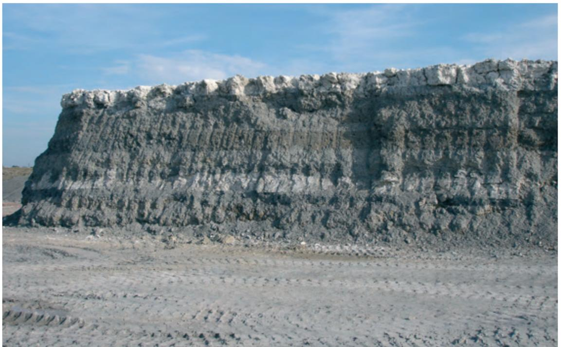
*Blending fireclays using layered stockpiles.*
